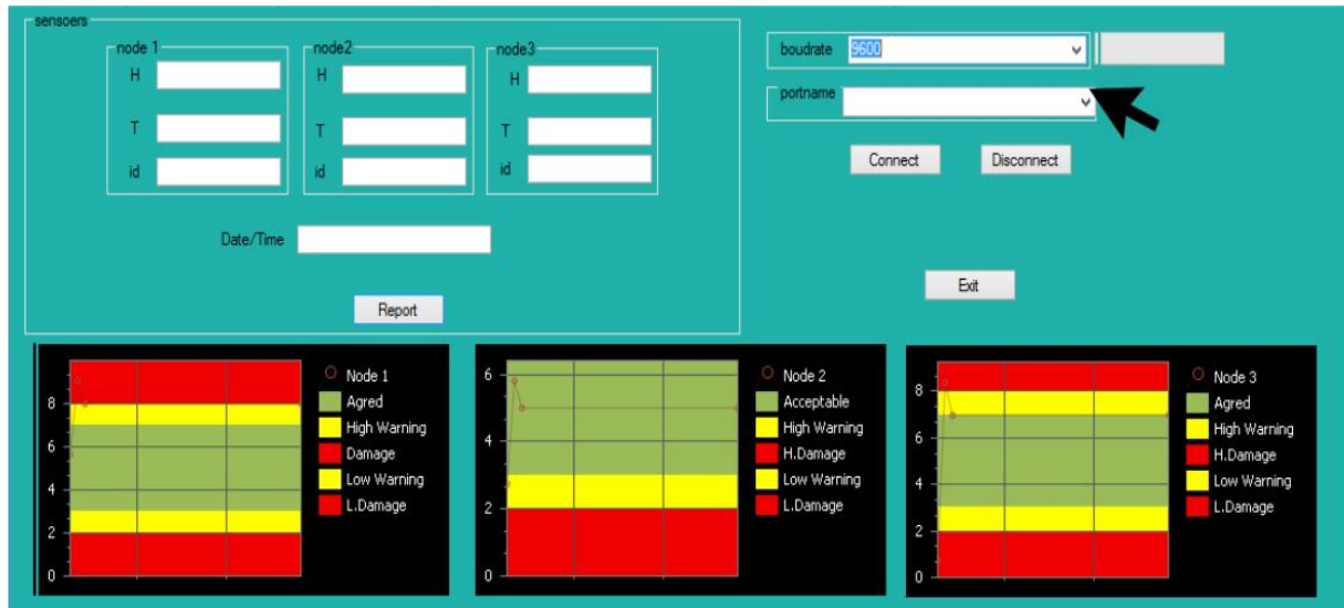
Fig (6.3) choose baud rate for data transmission.
