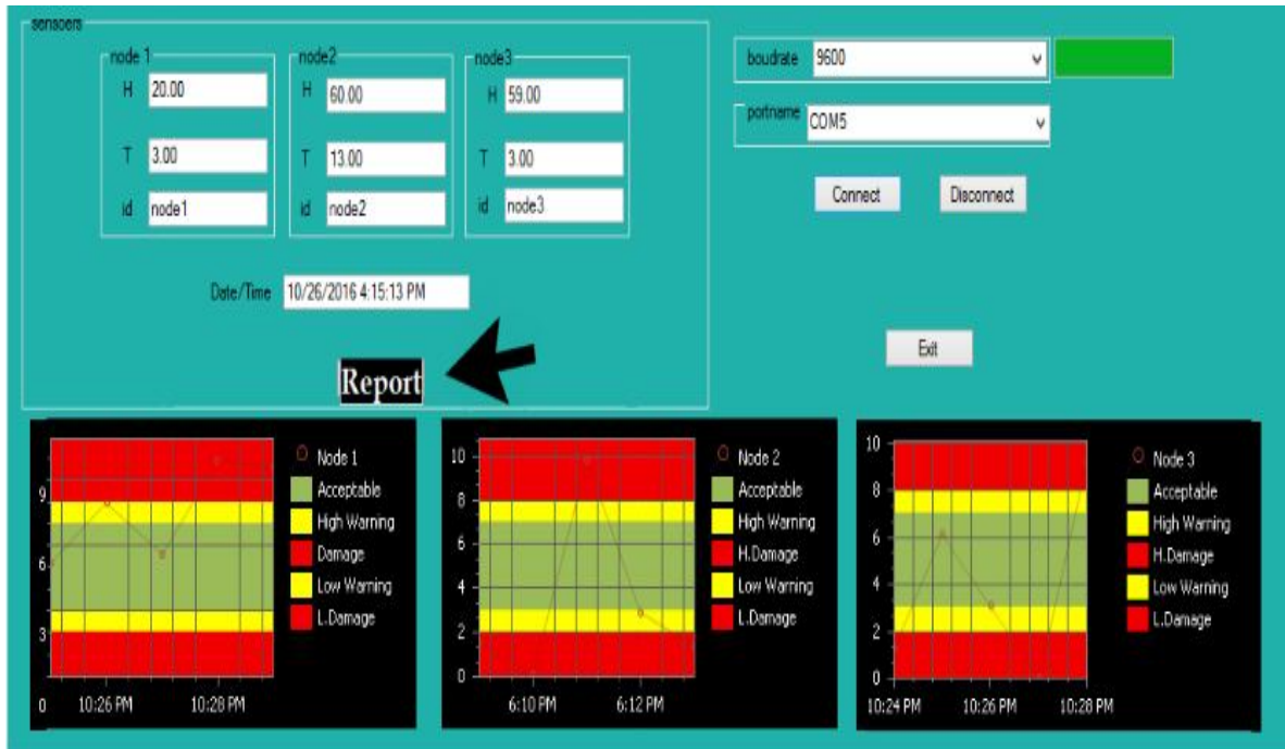
Fig(6.9) generates report for the stored sensors 'nodes parameters.
