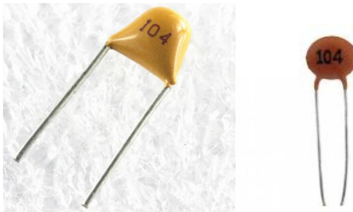
Fig 4.8 capacitor used to complete the low pass filter [21].
