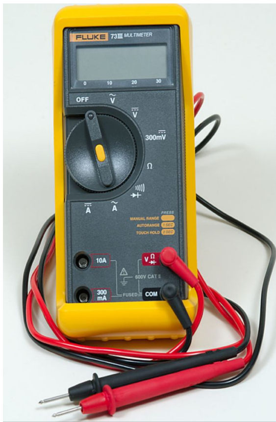
Fig .4.12 Fluke digital multimeter that measures current, voltage, resistance and capacitance in both DC and AC
