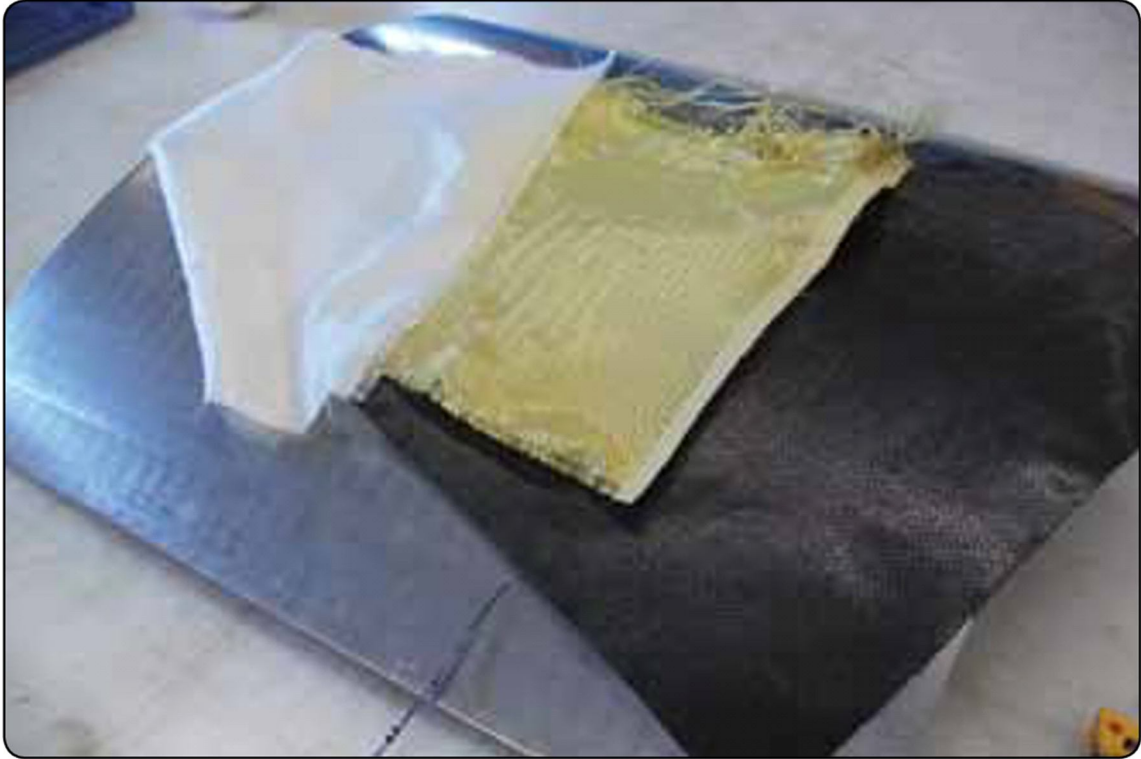
Figure 4 Fiberglass (left), Kevlar (middle), and carbon fiber
