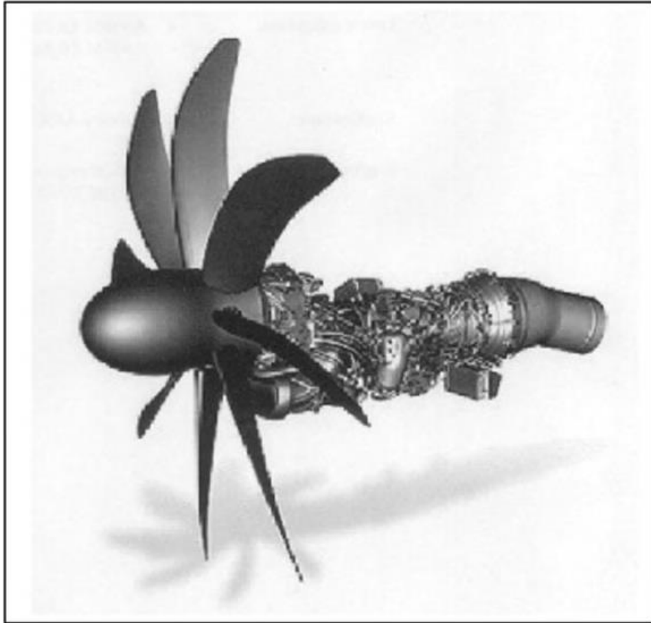
Figure 21. The Euro prop International TP 400 three-shaft turboprop engine with high-speed propeller.
