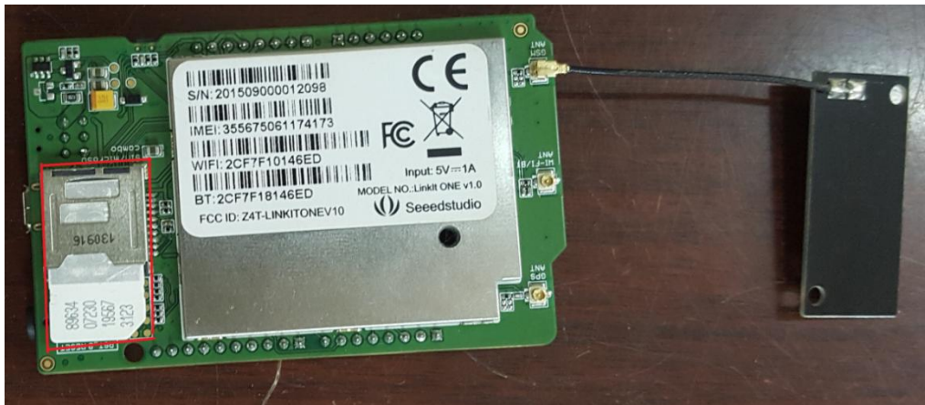
Figure 3.5: hardware setup of GPRS antenna and SIM card:
