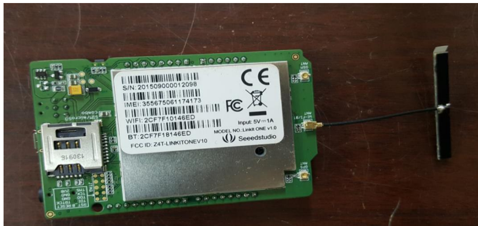
Figure 3.6: Wi-Fi antenna attached to the LinkIt-ONE
