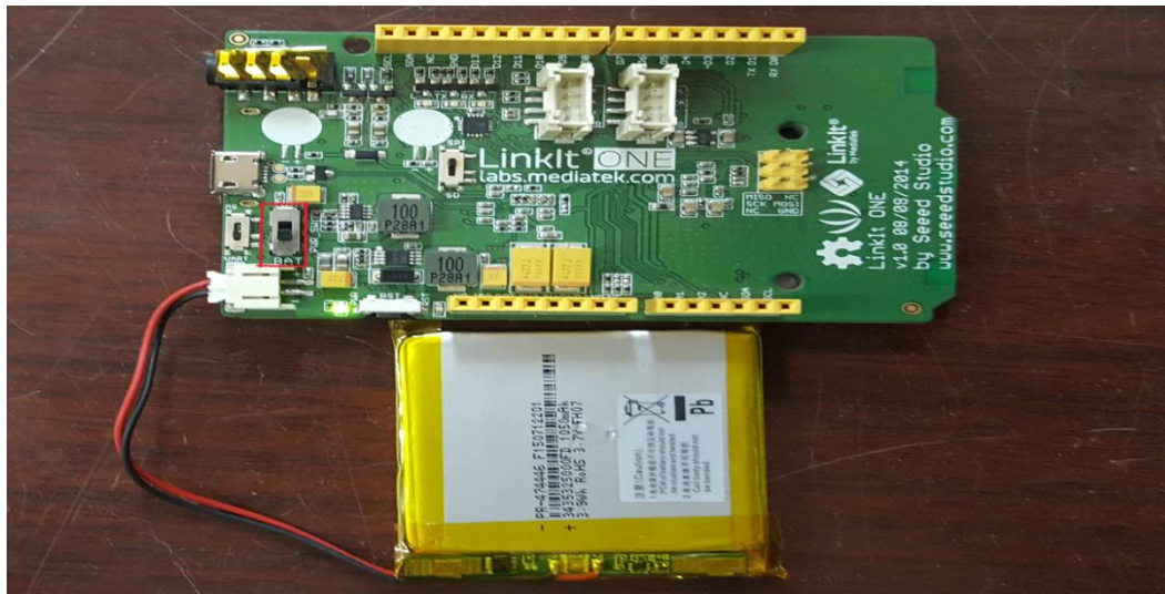
Figure 3.8: LinkitONE with battery source
