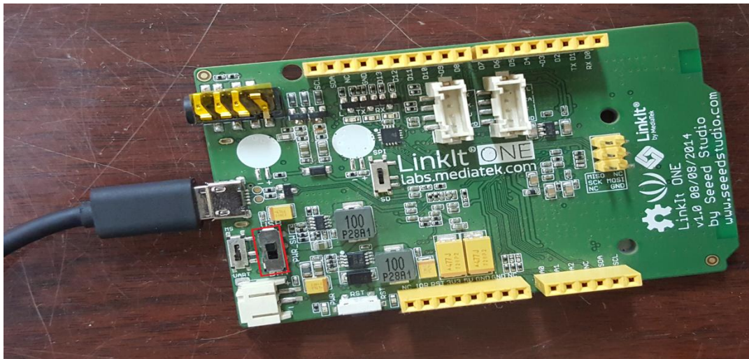
Figure 3.7: LinkitONE with USB power source:
