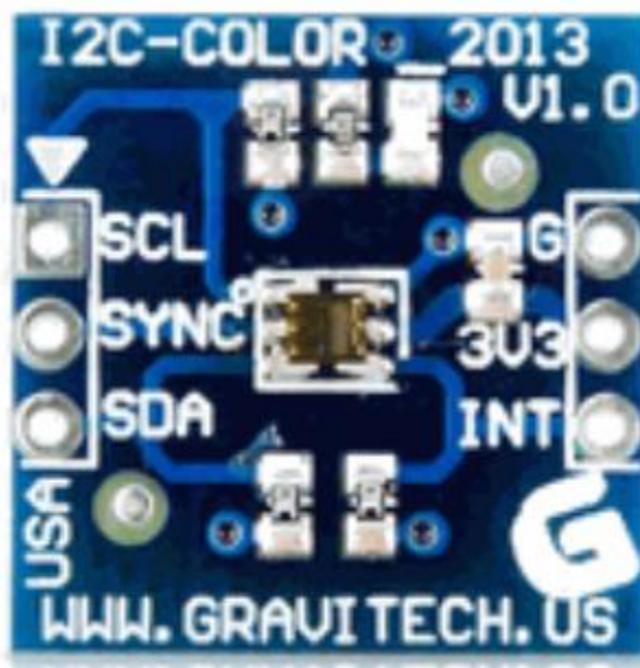
Figure 2.6: TCS3414CS color sensor.
