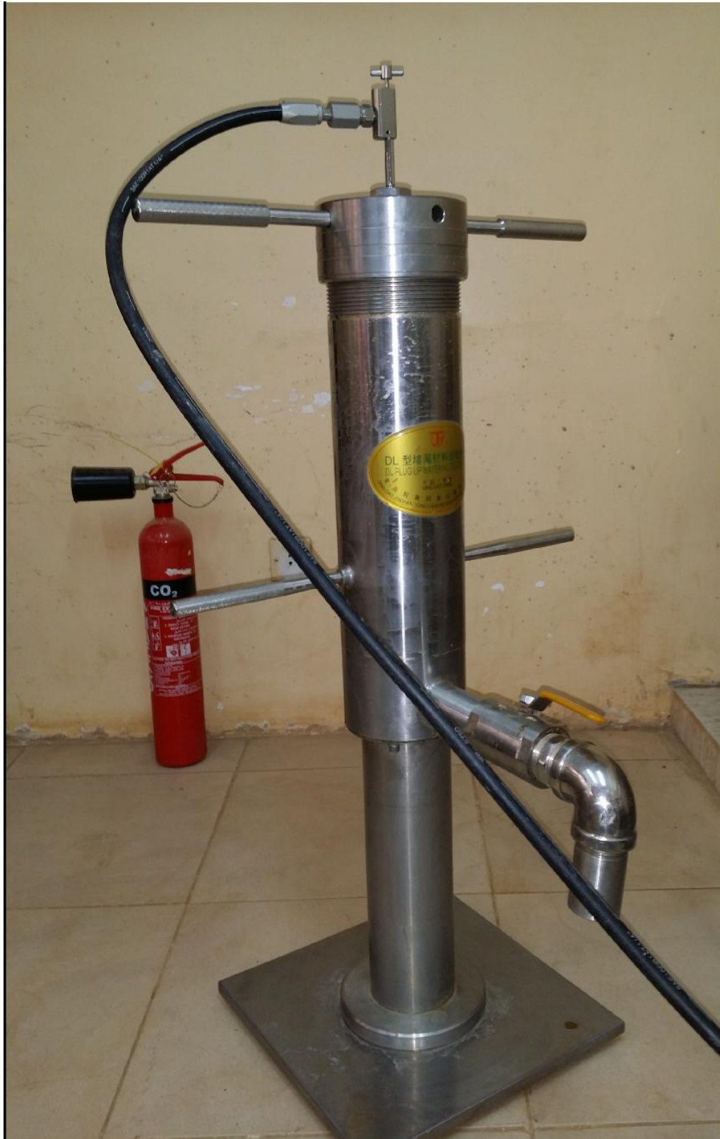
Figure (3-6): loss circulation device
