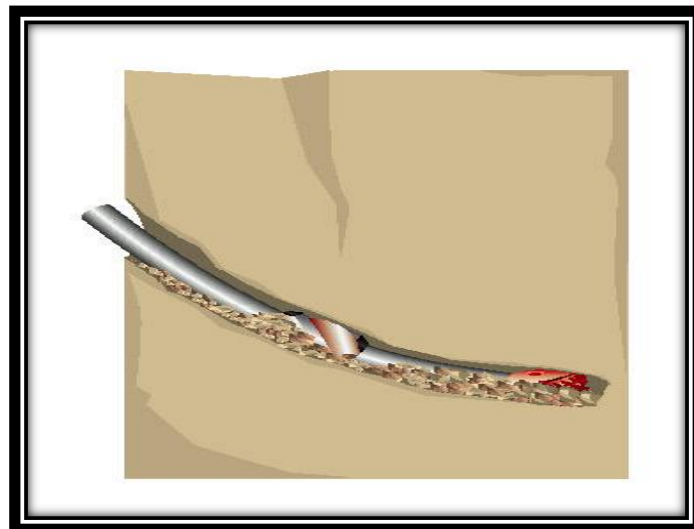
Fig(2-11) Poor cealing
