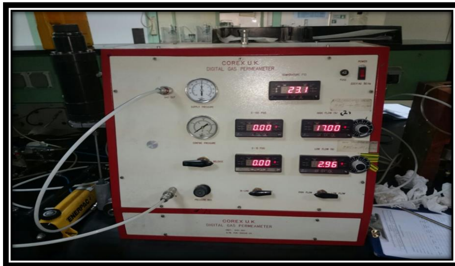
Fig.3-3 Digital gas permeameter device
