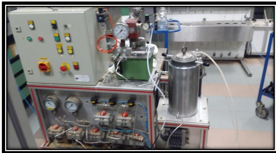
Fig.3.5 Automatic Saturator Machine
