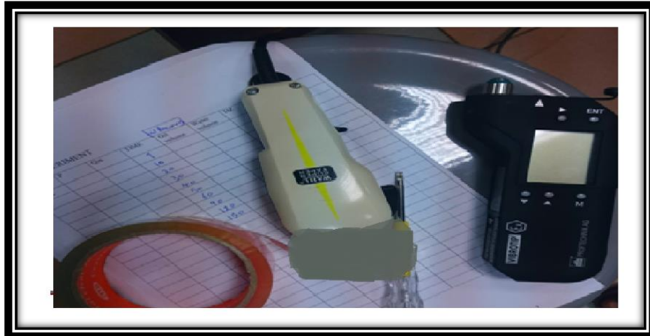
Fig.3-8 Vibration Generator and Vibration Measurement Devices.
