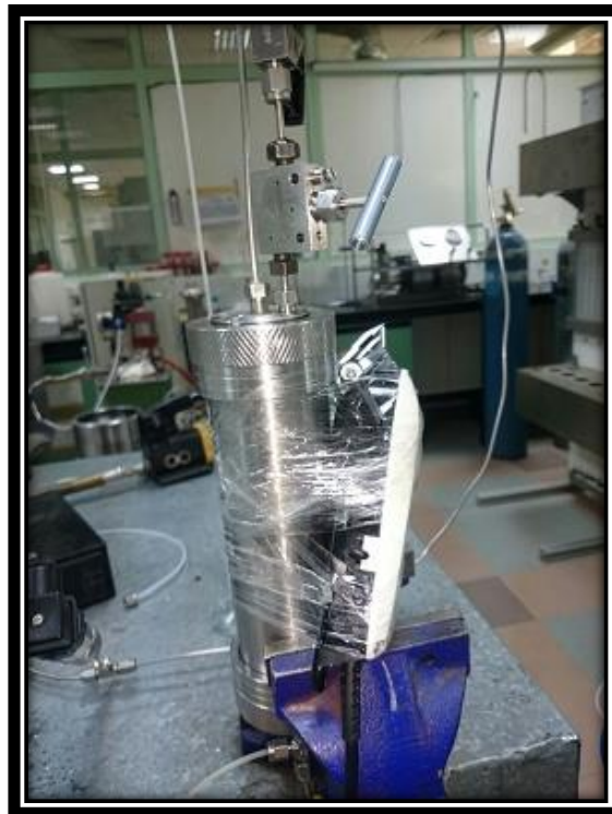
Fig. 3.9 Vibration Generator attached to Core Holder.
