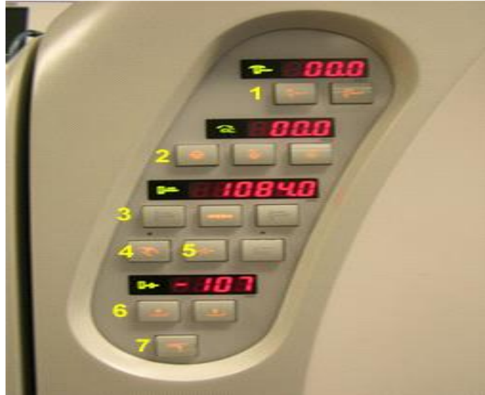
Figure (2-6): CT Gantry Control Panel
