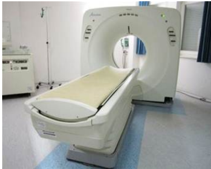
Figure (3.1) CT scan machine show gantry and couch
