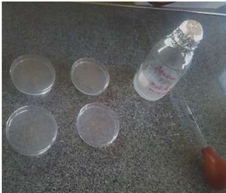
Figure 4. Preparation of the agarose gel for the agar gel precipitation/immunodiffusion test (AGPT/ AGID).
