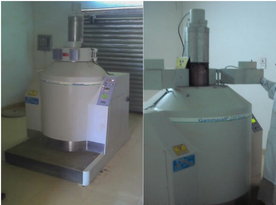
Figure 3.1 \gamma -irradiation cell models 220 at the national atomic energy research center- Khartoum
