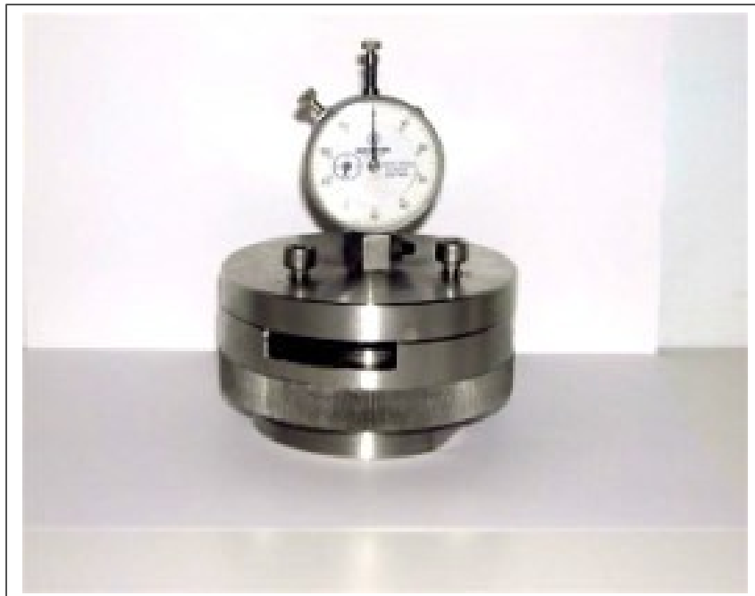
Fig 3.3 show E Type Universal Testing Machine used to determine the Load Deflection of polymer samples
