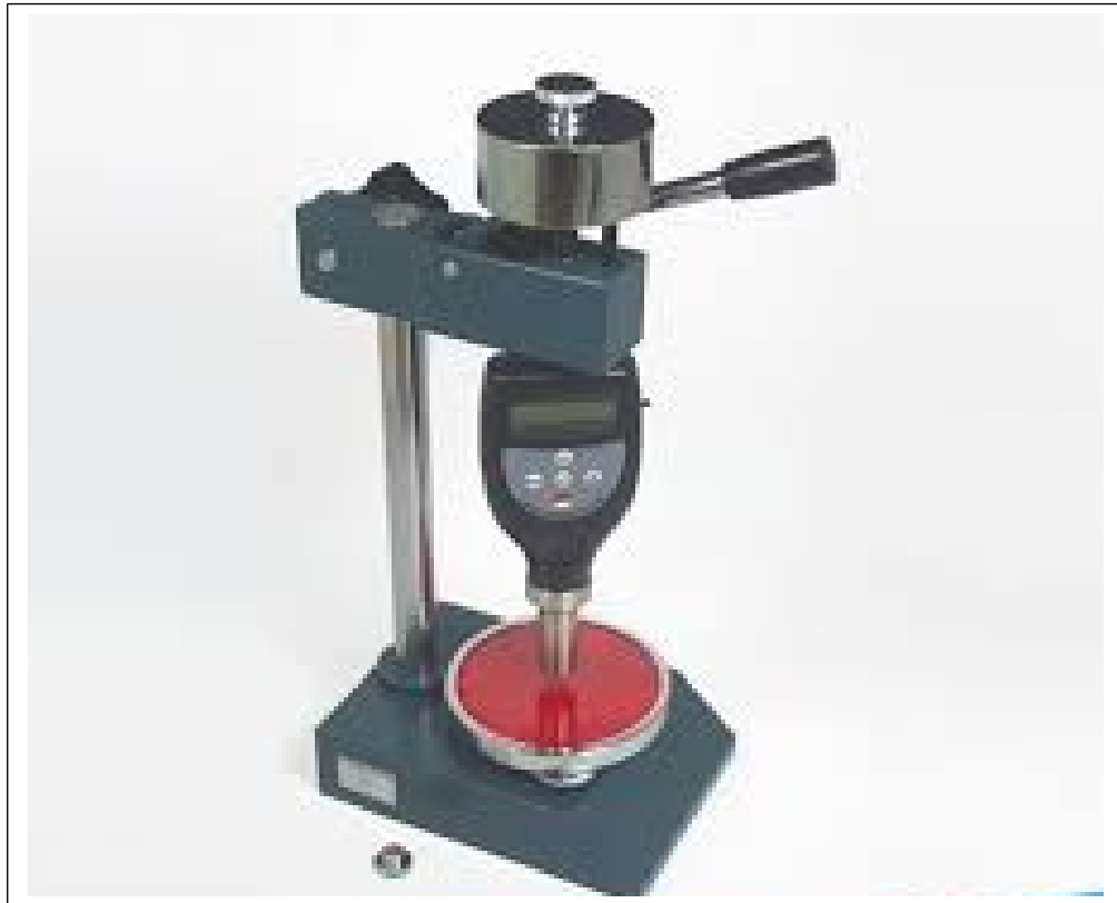
Fig 3.4 Zwick Roell Type A Durometer used to determine the Hardness of irradiated polymer samples.
