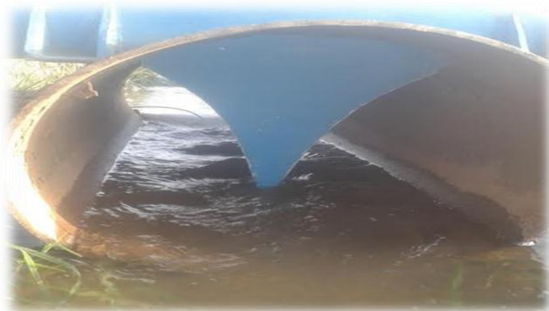
Figure (2.4) vane flow meter for determining flow rate
