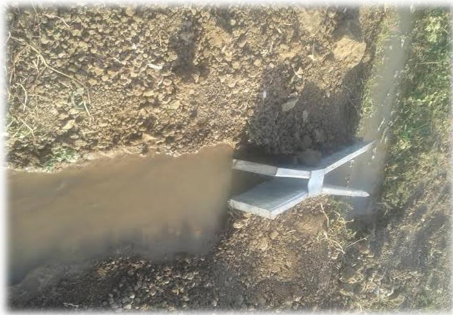
Figure (2.5): Parshal flume when determining flow rate
