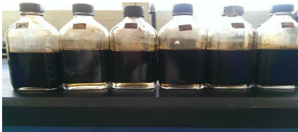
Fig. 3.17 Water separation of HJ.P10 at five different concentrations at 60°C after 24 hours
