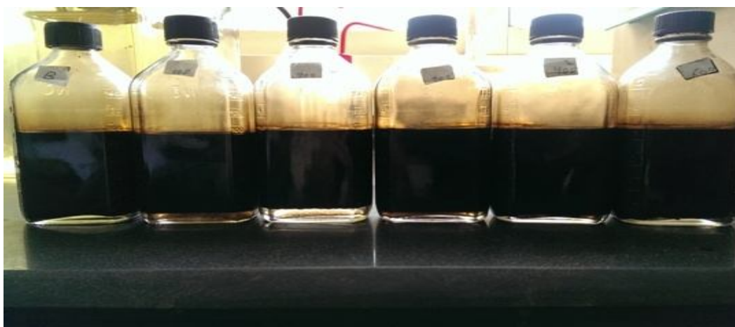
Fig. 3.25 Water separation of RHJ.E10 at five different concentrations at 60°C after 24 hours
