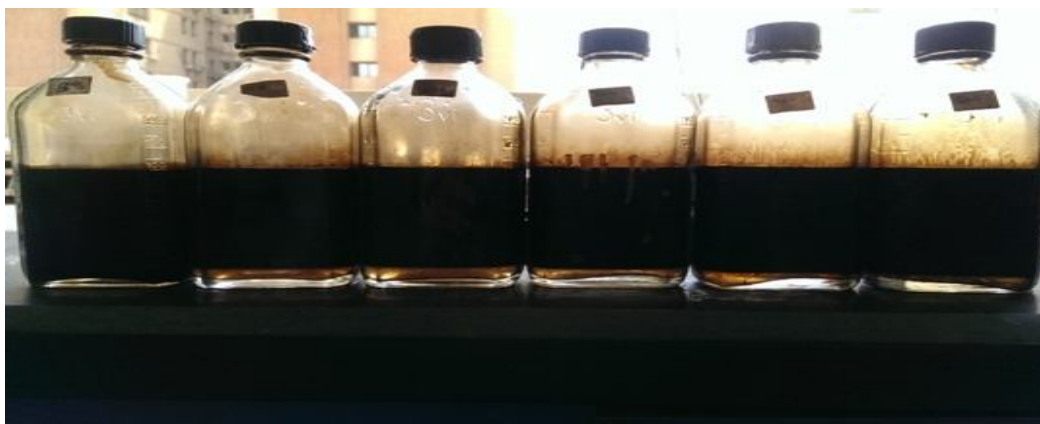
Fig. 3.19 Water separation of HJ.P30 at five different concentrations at 60°C after 24 hours
