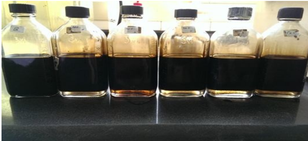
Fig. 3.21 Water separation of OHJ.E30 at five different concentrations at 60°C after 24 hours
