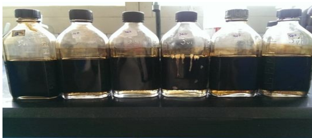
Fig. 3.16 Water separation of HJ.E30 at five different concentrations at 60°C after 24 hours
