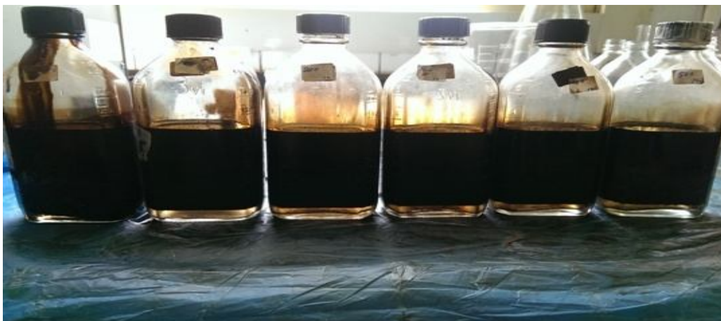
Fig. 3.22 Water separation of OHJ.P10 at five different concentrations at 60°C after 24 hours
