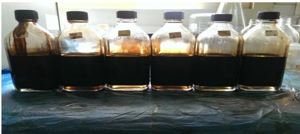
Fig. 3.23 Water separation of OHJ.P20 at five different concentrations at 60°C after 24 hours
