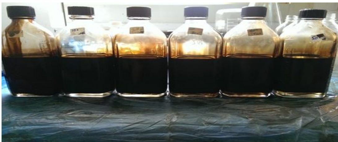
Fig. 3.26 Water separation of RHJ.E20 at five different concentrations at 60°C after 24 hours
