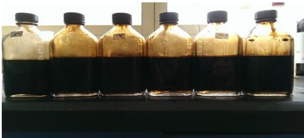
Fig. 3.29 Water separation of RHJ.P20 at five different concentrations at 60°C after 24 hours
