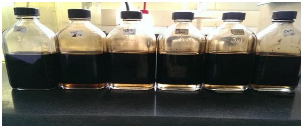
Fig. 3.24 Water separation of OHJ.P30 at five different concentrations at 60°C after 24 hours
