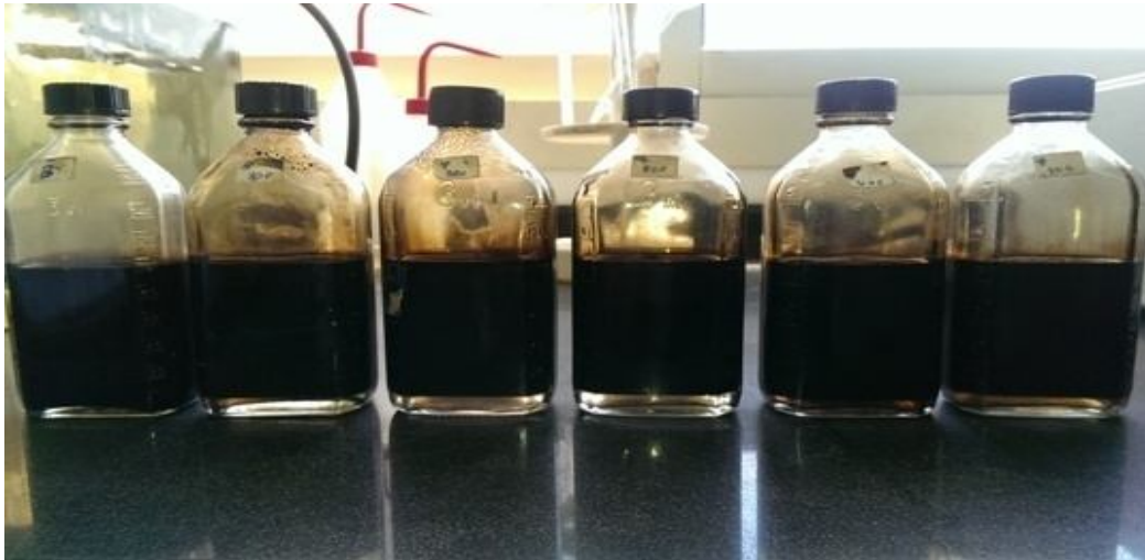
Fig. 3.30 Water separation of RHJ.P30 at five different concentrations at 60°C after 24 hours
