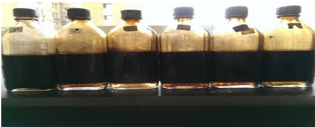
Fig. 3.20 Water separation of OHJ.E20 at five different concentrations at 60°C after 24 hours
