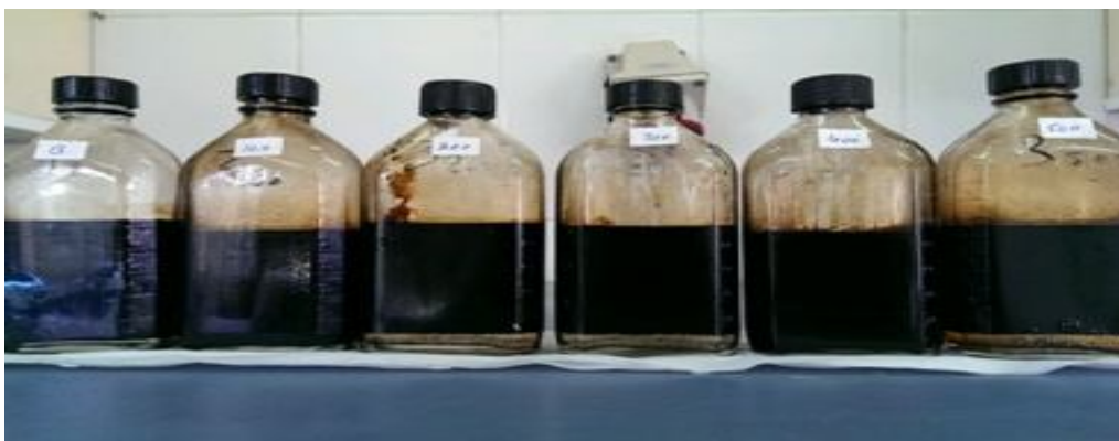
Fig. 3.14 Water separation of HJ.E10 at five different concentrations at 60°C after 24 hours
