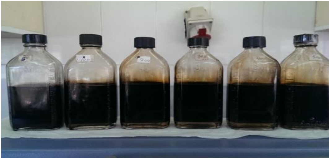
Fig. 3.27 Water separation of RHJ.E30 at five different concentrations at 60°C after 24 hours
