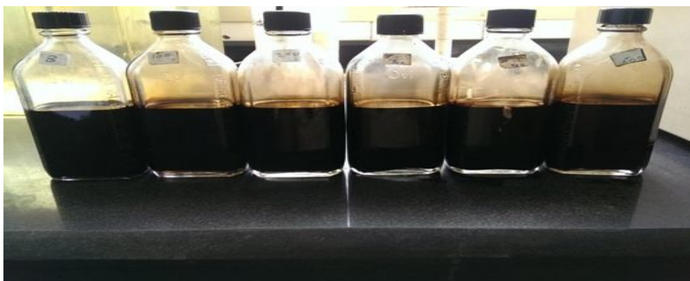
Fig. 3.15 Water separation of HJ.E20 at five different concentrations at 60°C after 24 hours
