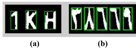
Figure 6.1: The Input to LP Character Recognition Stage (a) English Characters Image. (b) Indian Numbers Image.
