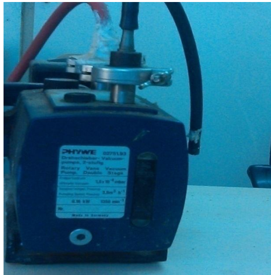
Figure (3-2): A photograph of the vacuum pump.
