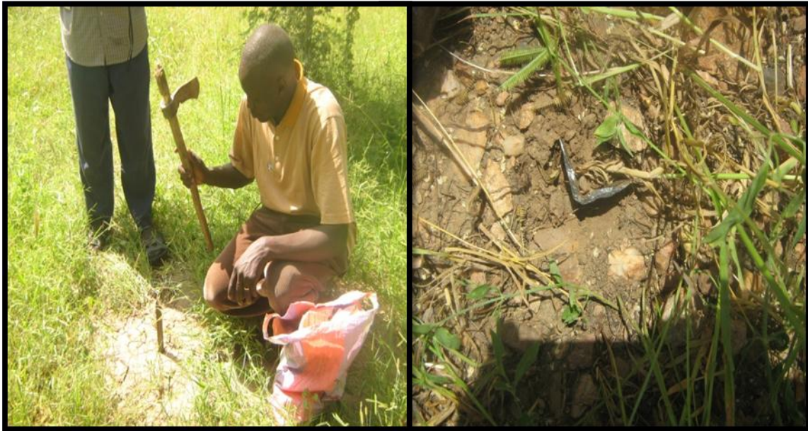
Plate. 15. The process of fixing metal pegs in the center of sample plot at the left and metal pegs after fixed at the right.
