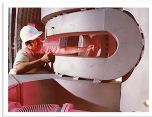
Figure (1.2) showing Magnetic mirrors suffered from end losses, requiring high power, complex magnetic designs, such as the baseball coil pictured here.
