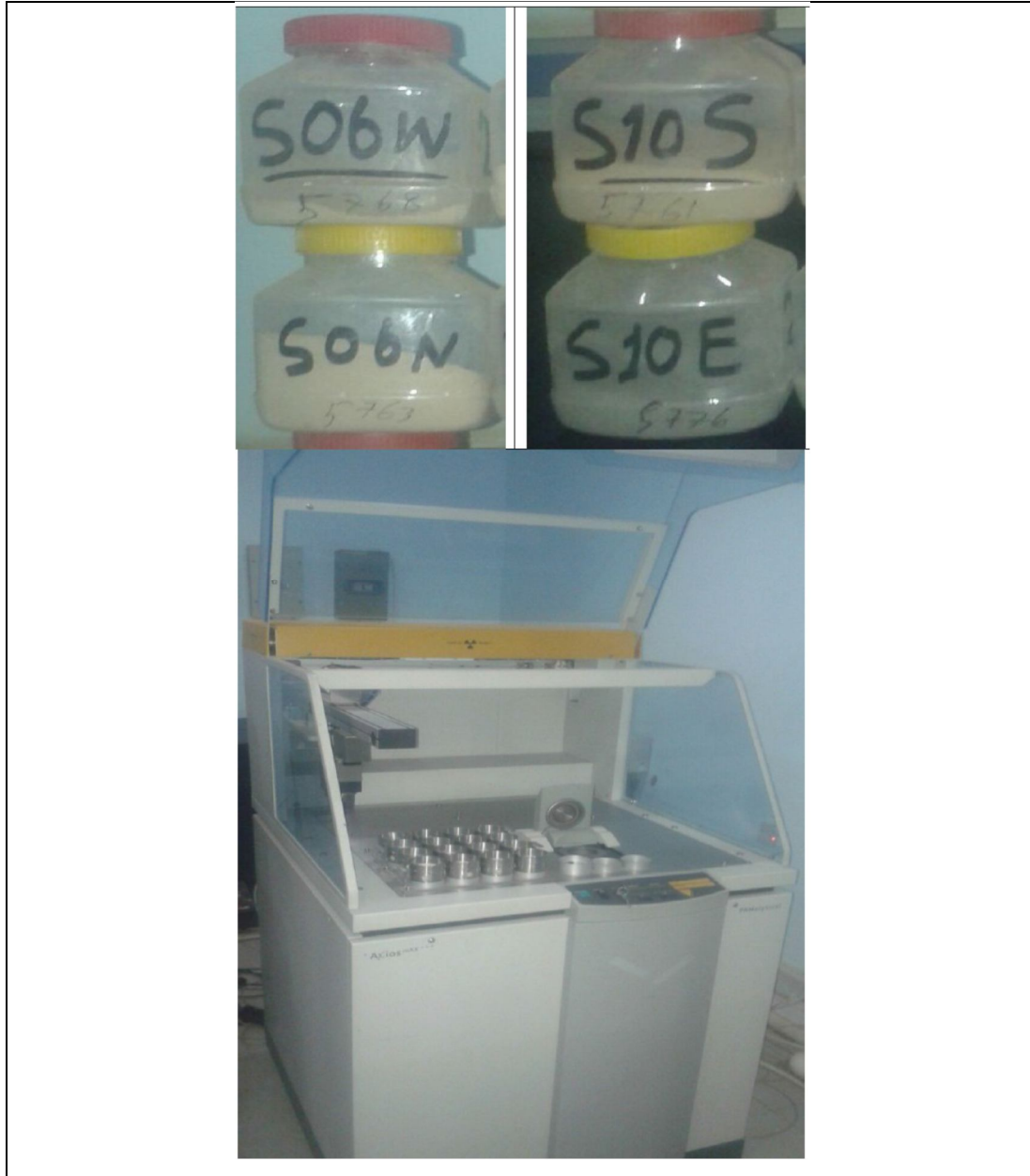
Figure 4.2: sample sealed and transferred to a plastic container of 200g
