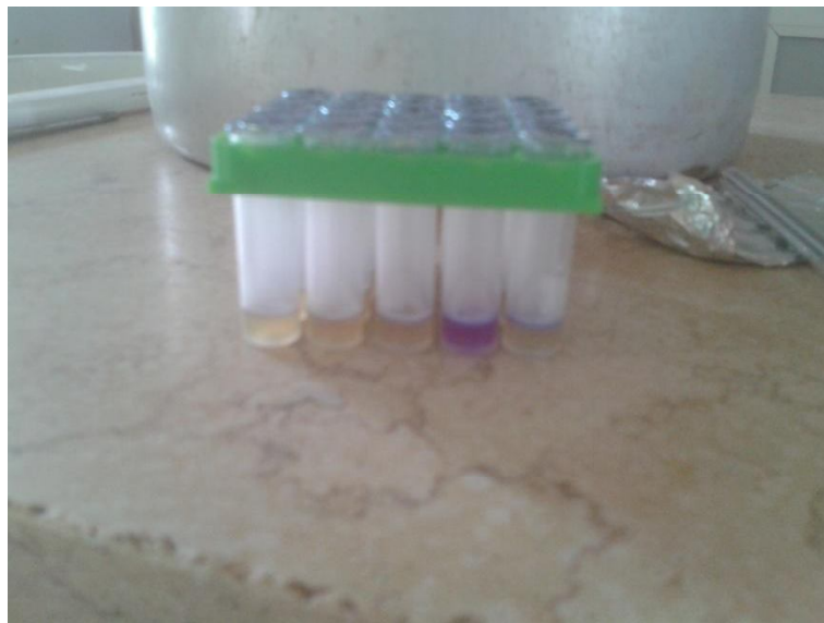
Figure 3.2: Delvotest result after 3 hr. incubation period ( yellow color indicates –ve result and purple color indicates +ve color).
