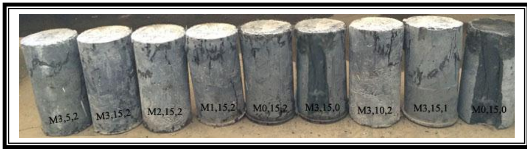
Plate 3.6: Compression Failure of NSRPC Cylinders
