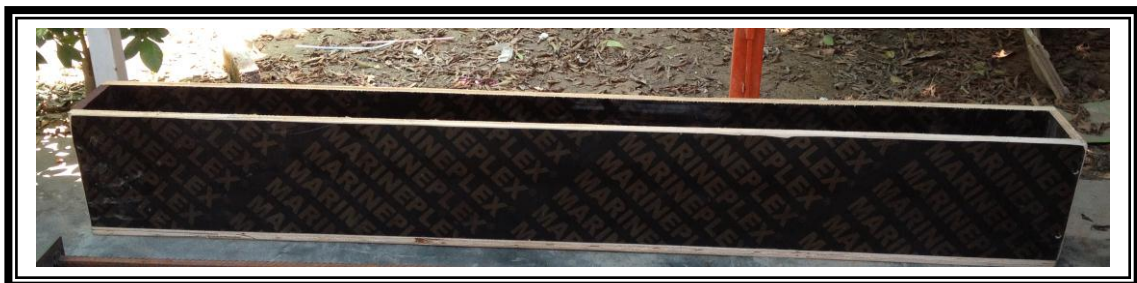
Plate 3.2: The Wooden Molds Used in Casting NSRPC Beams
