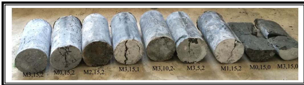
Plate 3.7: Tensile Splitting Failure of NSRPC Cylinders
