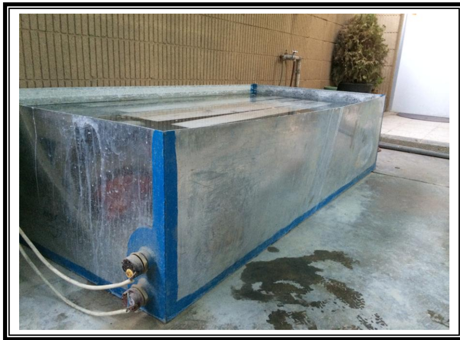
Plate 3.3: Curing of Specimens
