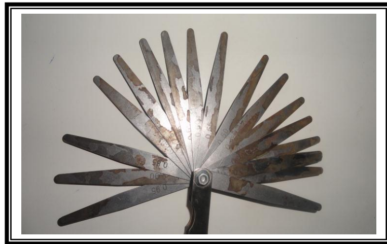
Plate 3.11: Set of Plates Used for Measuring the Crack Width
