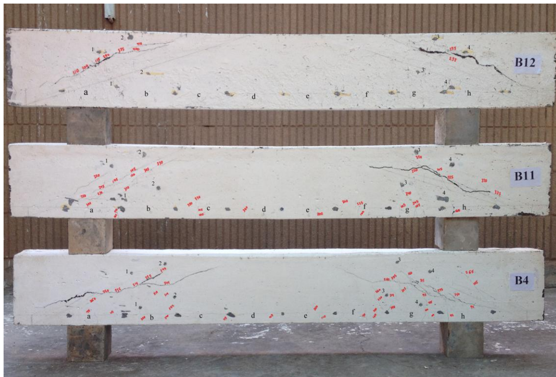
Plate 4.5A Crack Patterns of NSRPC Beams (B4,B11,B12 with Varying a/d, V_f=2\% )
