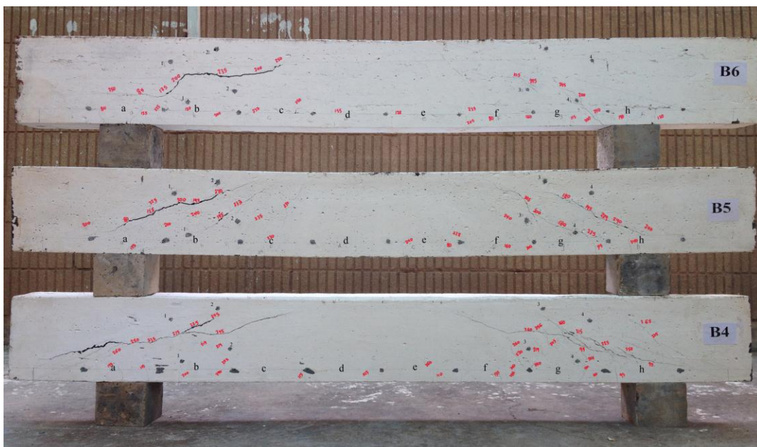
Plate 4.2 Crack Patterns of NSRPC Beams (B5,B6,B4 with Varying SF)
