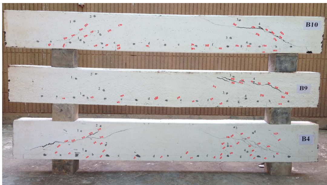
Plate 4.4 Crack Patterns of NSRPC Beams (B4,B9,B10 with Varying \rho )
