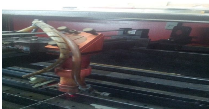
Fig (3.6): Technique of deliver laser beam to working area by mirrors.
