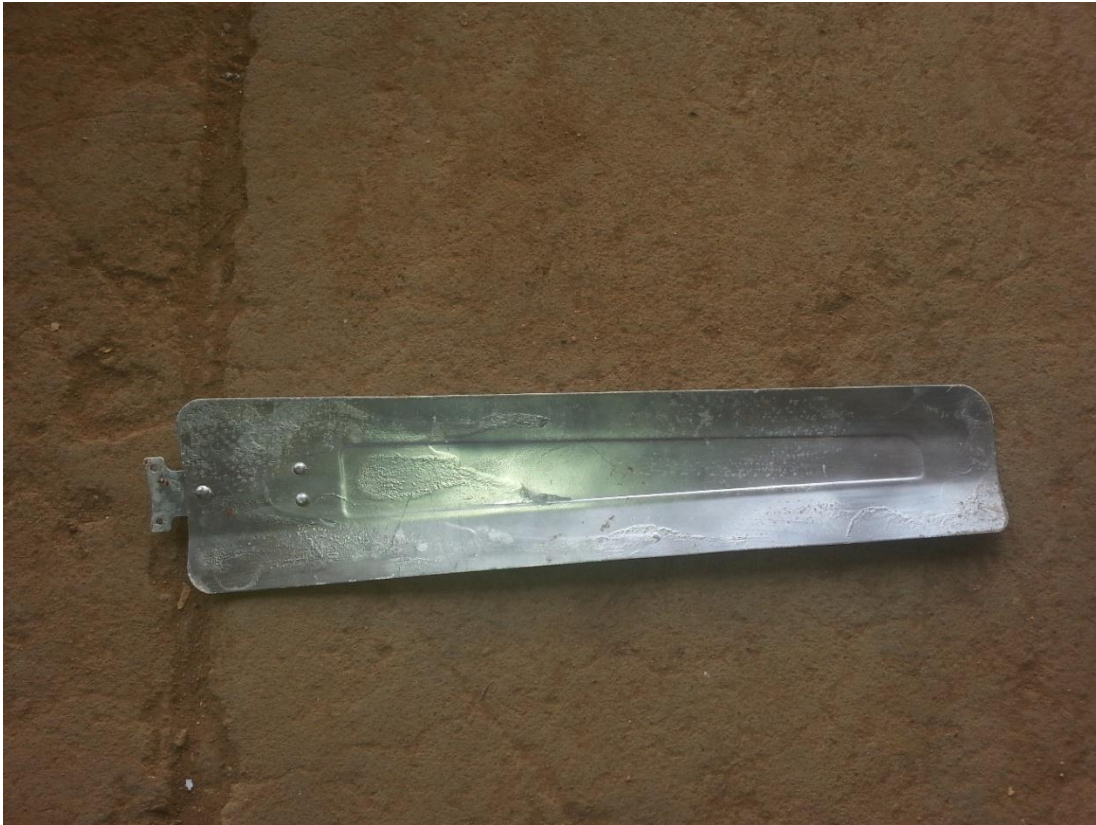
Figure (3.1) show the blade of wind turbine
