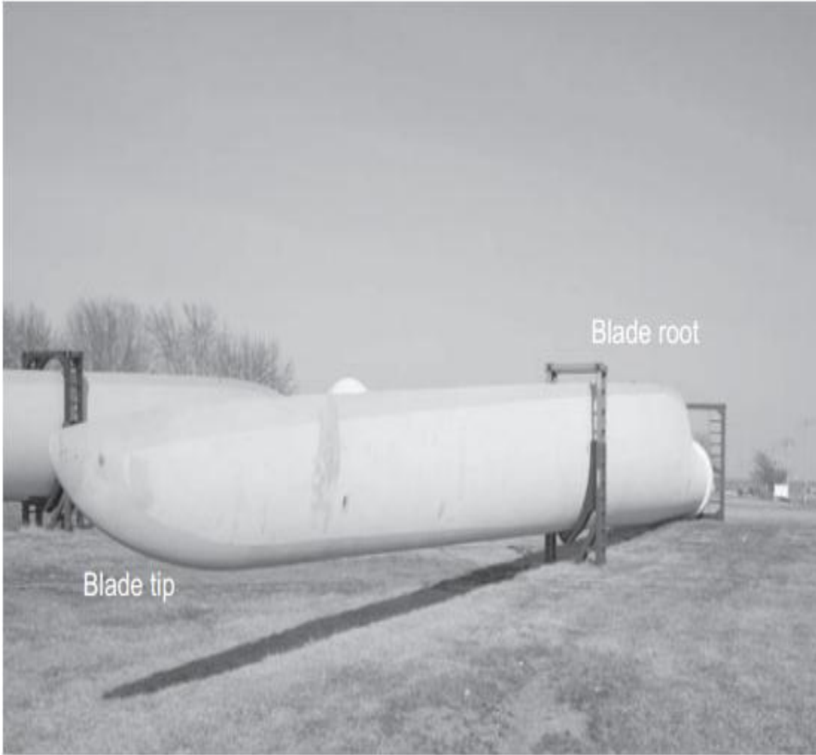
Figure (2.17) a typical blade of a modern wind turbine.
