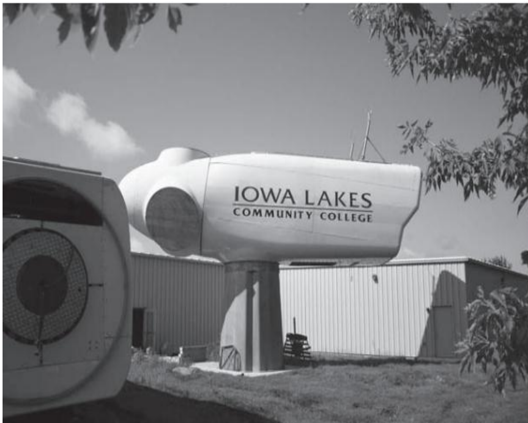
Figure (2.15) show the nacelle and hub
