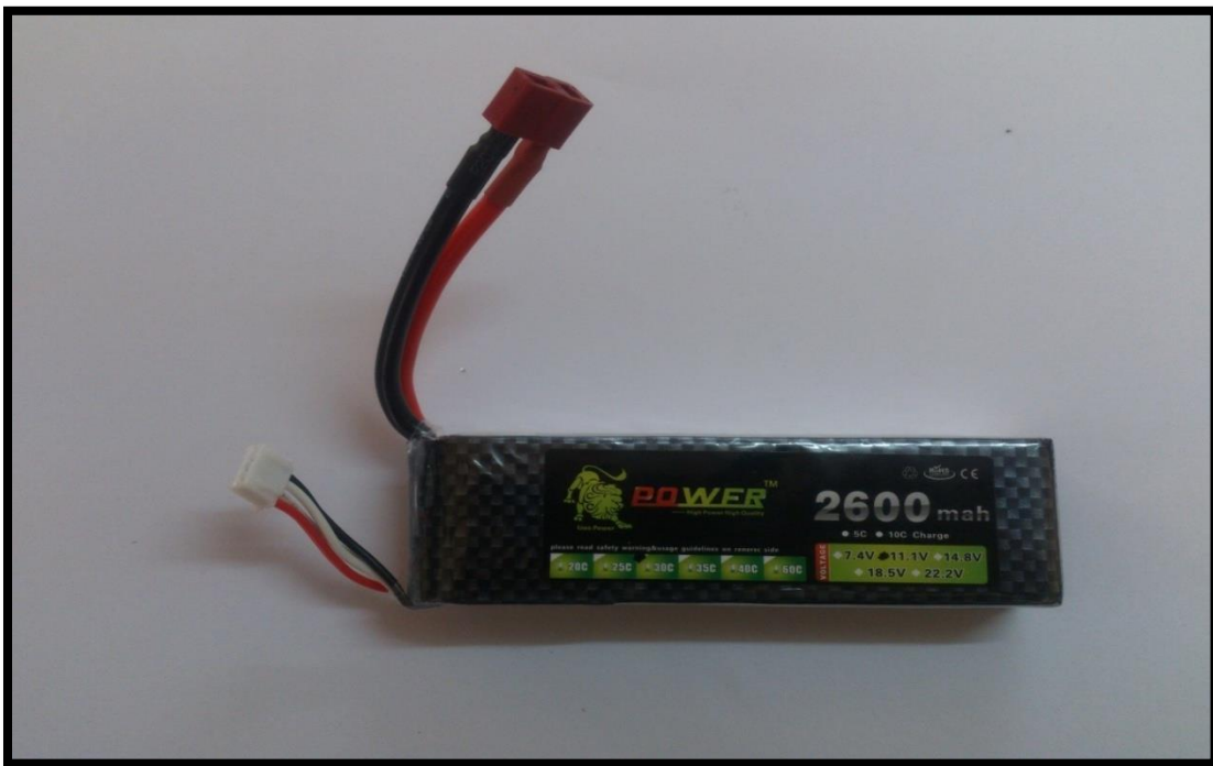
Figure 3-13: LiPo batteries 3S 11.1V 2600MAH 30C packs
