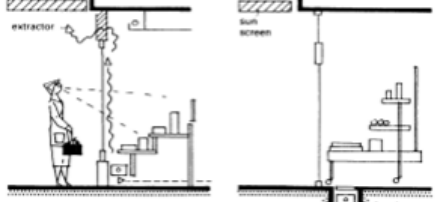
8 Stepped window display, with protective glass behind
