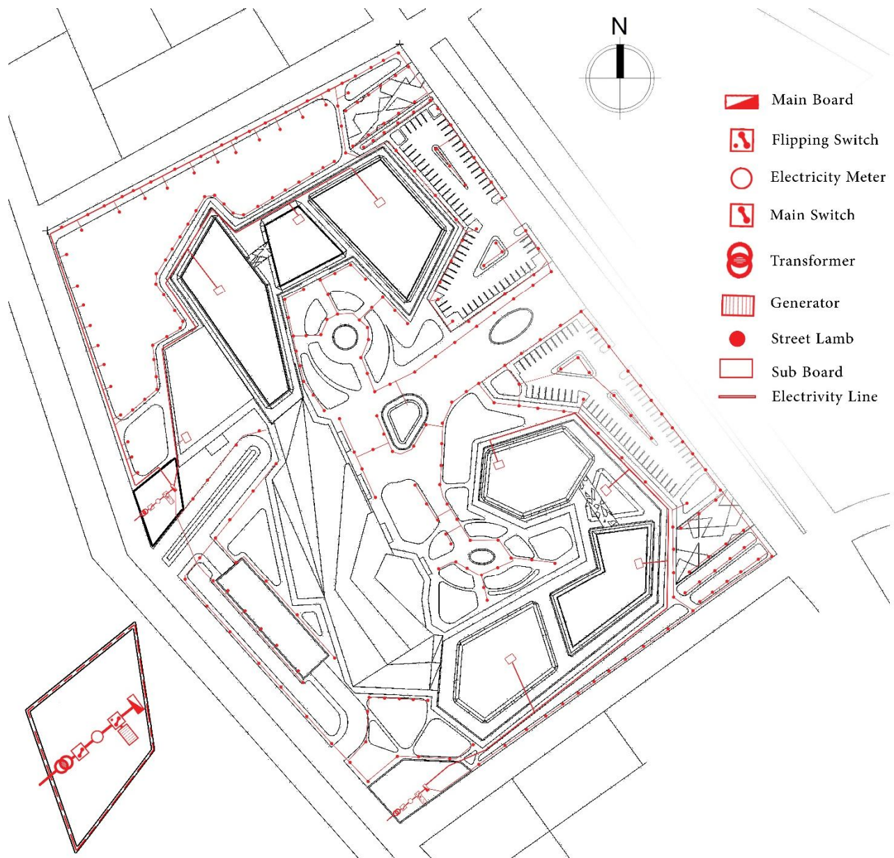
Figure 67: Site plan to showcase the electricity lines in the project with a part plan of one of the two generators room.
