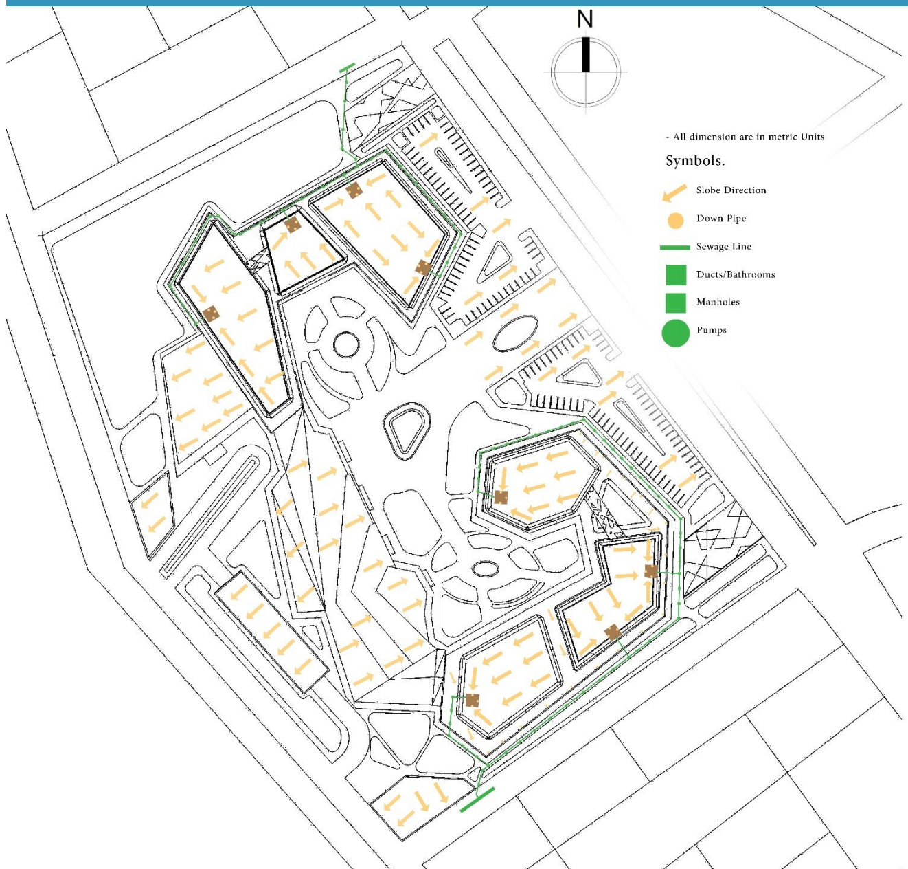
Figure 65: Site Plan showcasing how the sewage system and the drainage system are working.
