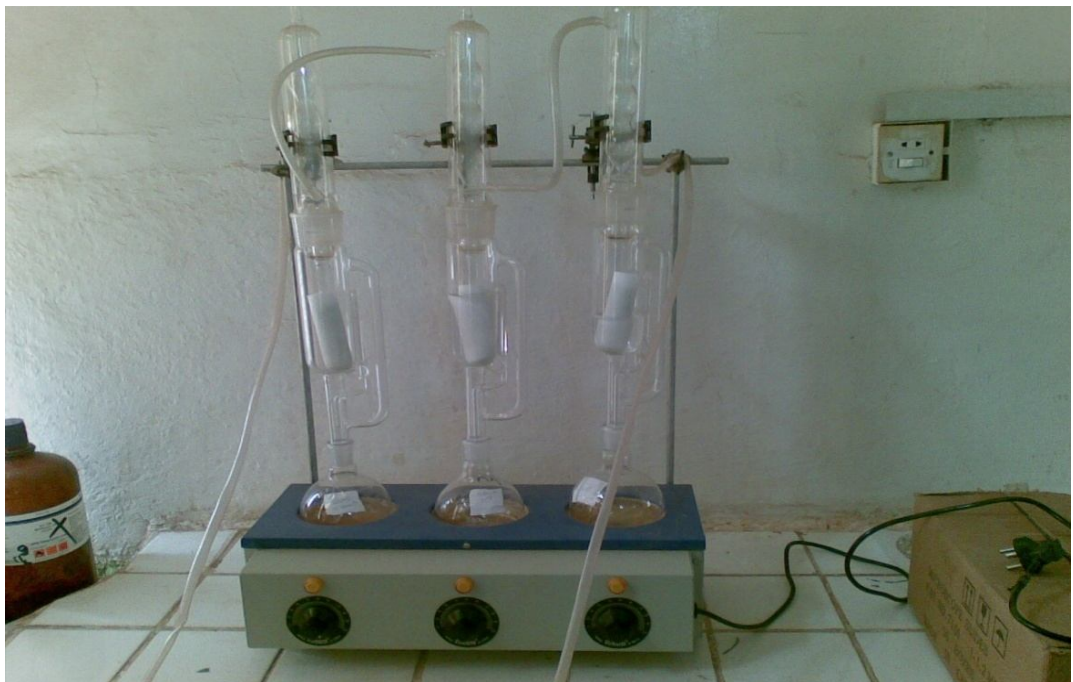
Plate 9: Soxhlet for extraction Apparatus
