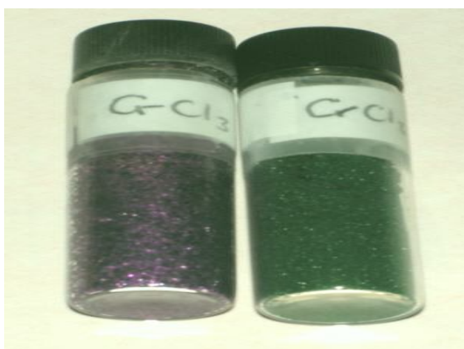
Scheme 1.1.: Anhydrous CrCl 3 and hydrated "CrCl 3 .6H 2 O",
