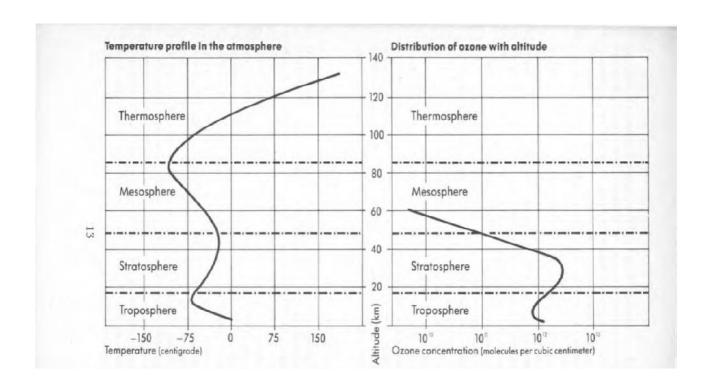
Figure 1.1 The layered structure of the atmosphere is shown by temperature profile ozone is concentrated in the stratosphere especial between 20 kmand30 km altitude .(source: present state of knowledge of the upper atmosphere NASA,1986).
