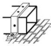
Install air ducts on the vertical walls
