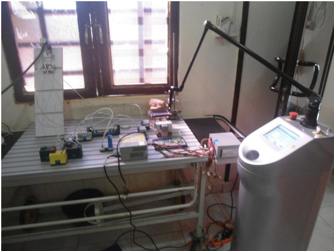
Figure 2.28 Final Experimental Setup for laser micromachining of PMMA
