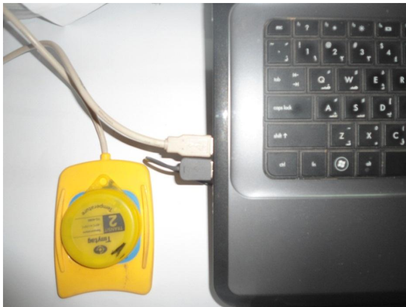
Figure 3.2 Inductive pad in connection with personal computer
