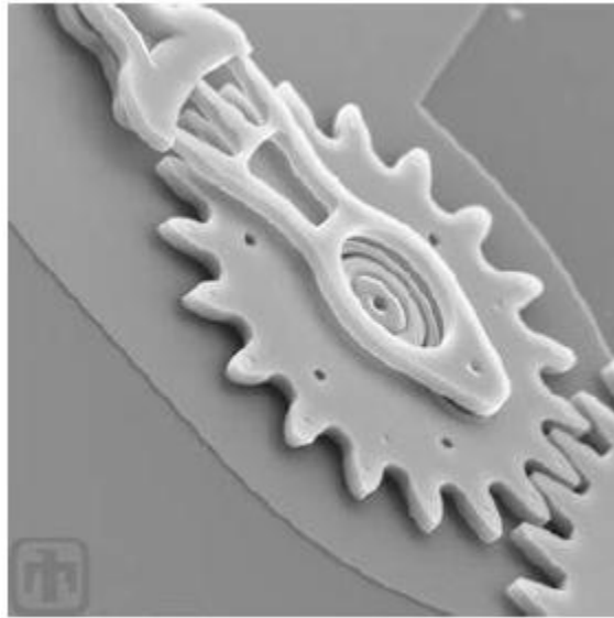
Figure 2.5: Micro-engine gear meshing with another gear
