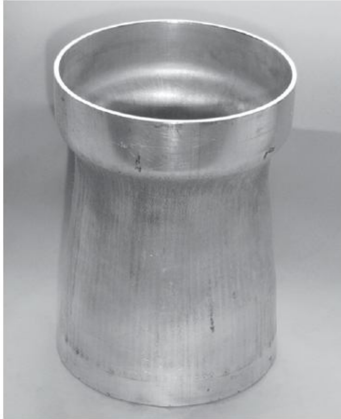
Figure 1.3 An example of laser bending being used to narrow a pipe while at the same time thickening the walls in the narrow section (Sarah Silve 2000).
