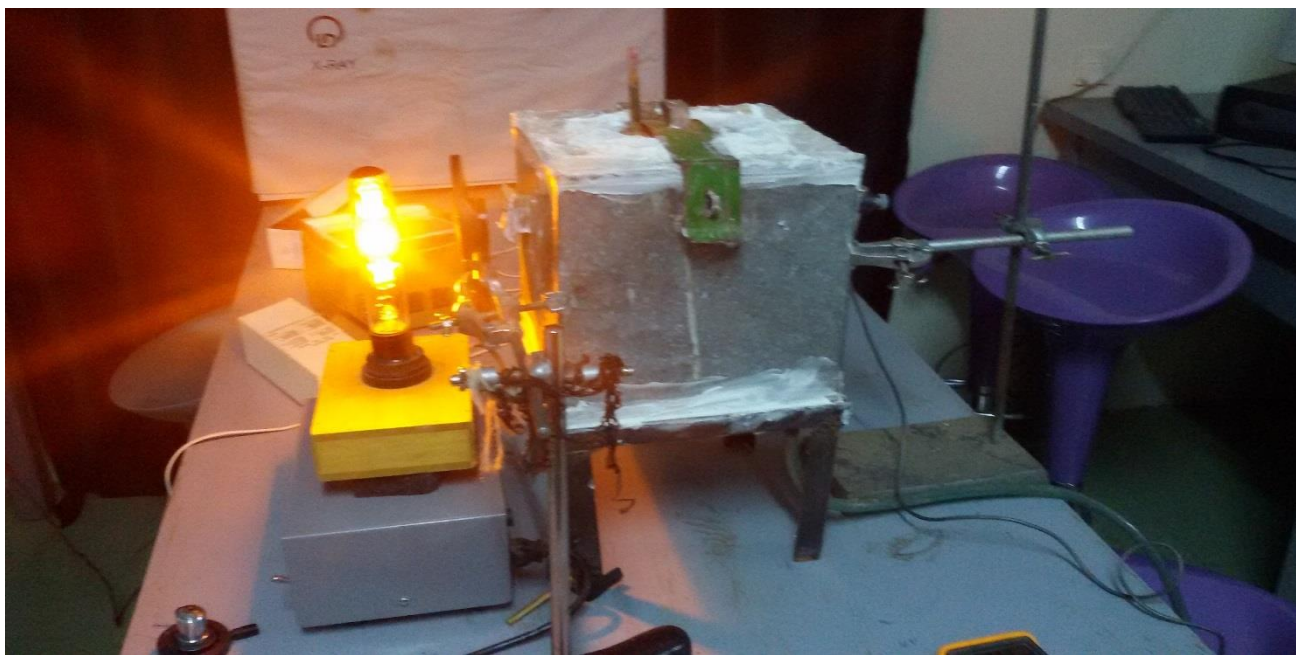
Fig.3.1: part of measurement of the transmitted intensity through the thin film using sodium light source
