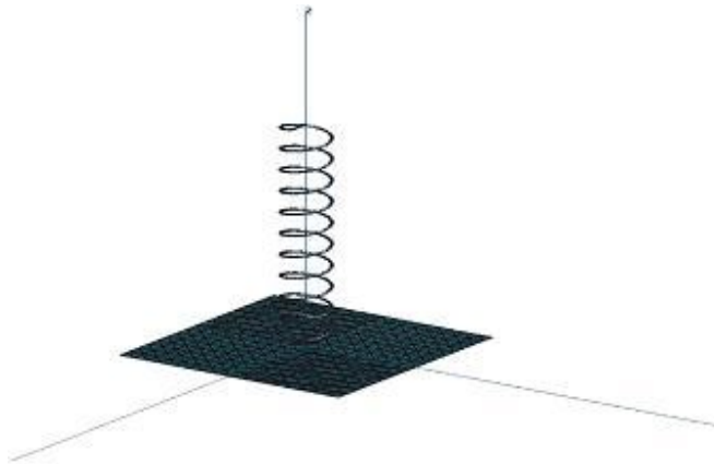
Figure (2.5) Structure of helical antenna
