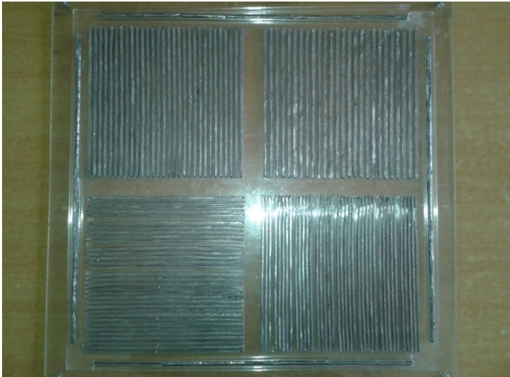
Figure 4-1: shows the frontal part of the phantom made of Perspex (42×42×10 cm) that simulates the four quadrant bars phantom each one was 20×20 cm.
