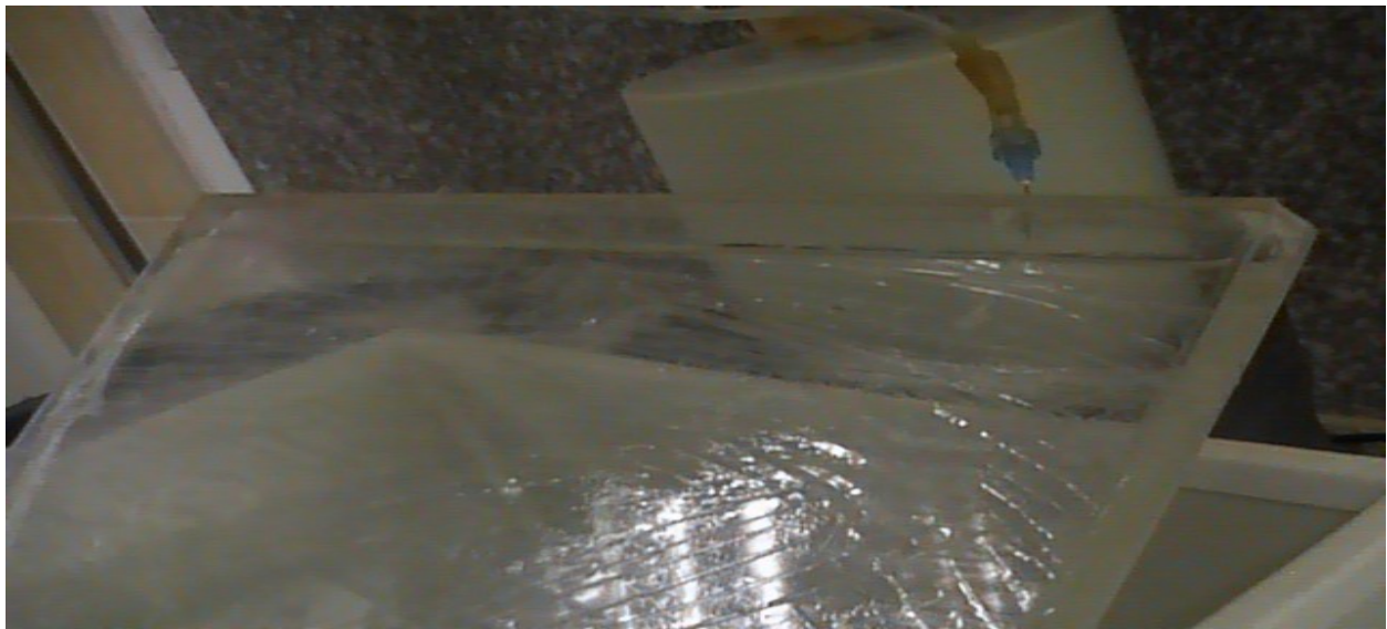
Figure 3-9: image show the flood phantom during filling with water (front view)
