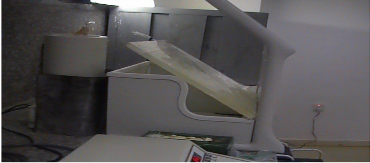
Figure 3-10: image show the flood phantom during filling with ^{99m}\text{Tc} (side view)
