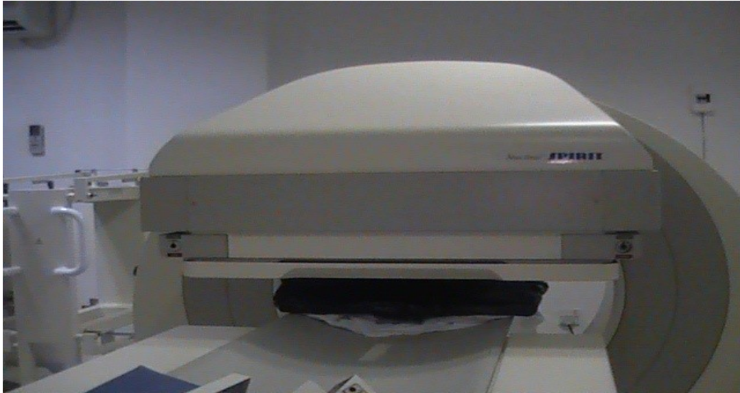
Figure 3-12: image show the flood phantom center during uniformity quality control test (front view)
