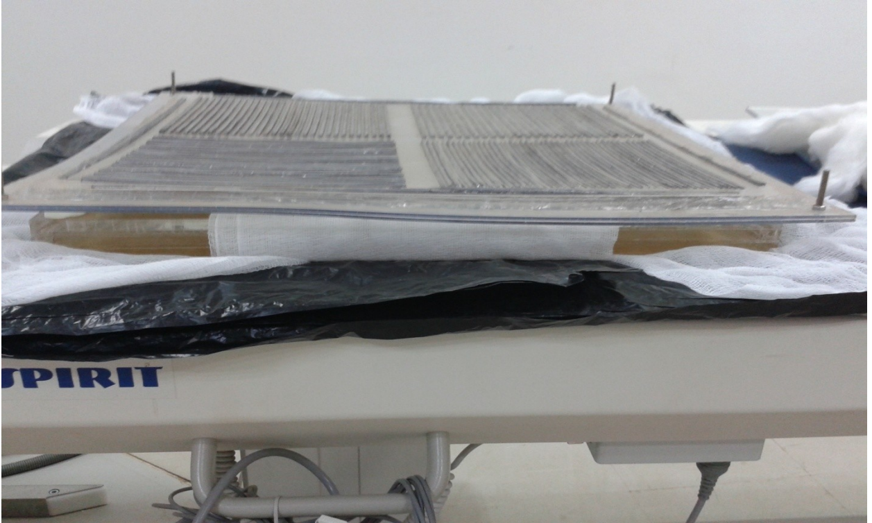
Figure 3-31: image shows the par phantom centering over the flood phantom (side view)
