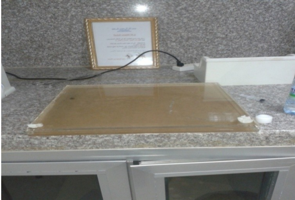
Figure 4-2: shows the back part simulates the liquid flood phantom made of Perspex (42×42×1 cm) and has orifice 0.5 cm to be fill with a liquid radioactive material
