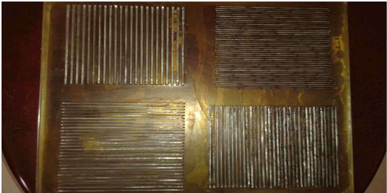
Figure 3-4: image show the lead within rubber sheet grooves of the bar quadrate phantom
