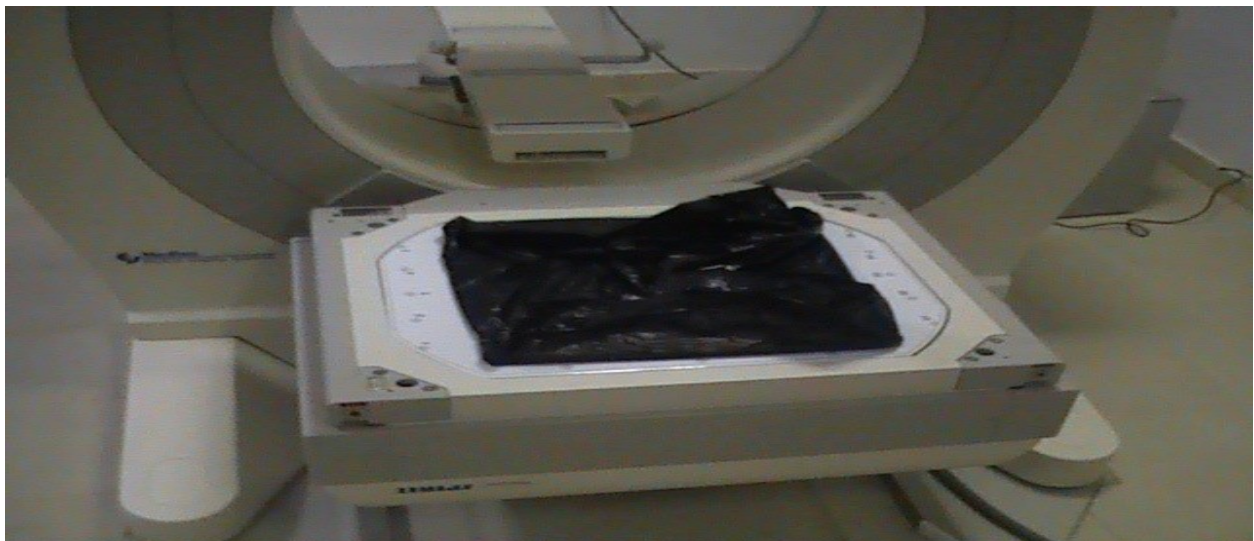
Figure 3-15: image show the bar quadrate phantom center during intrinsic linearity and resolution quality control test acquisition
