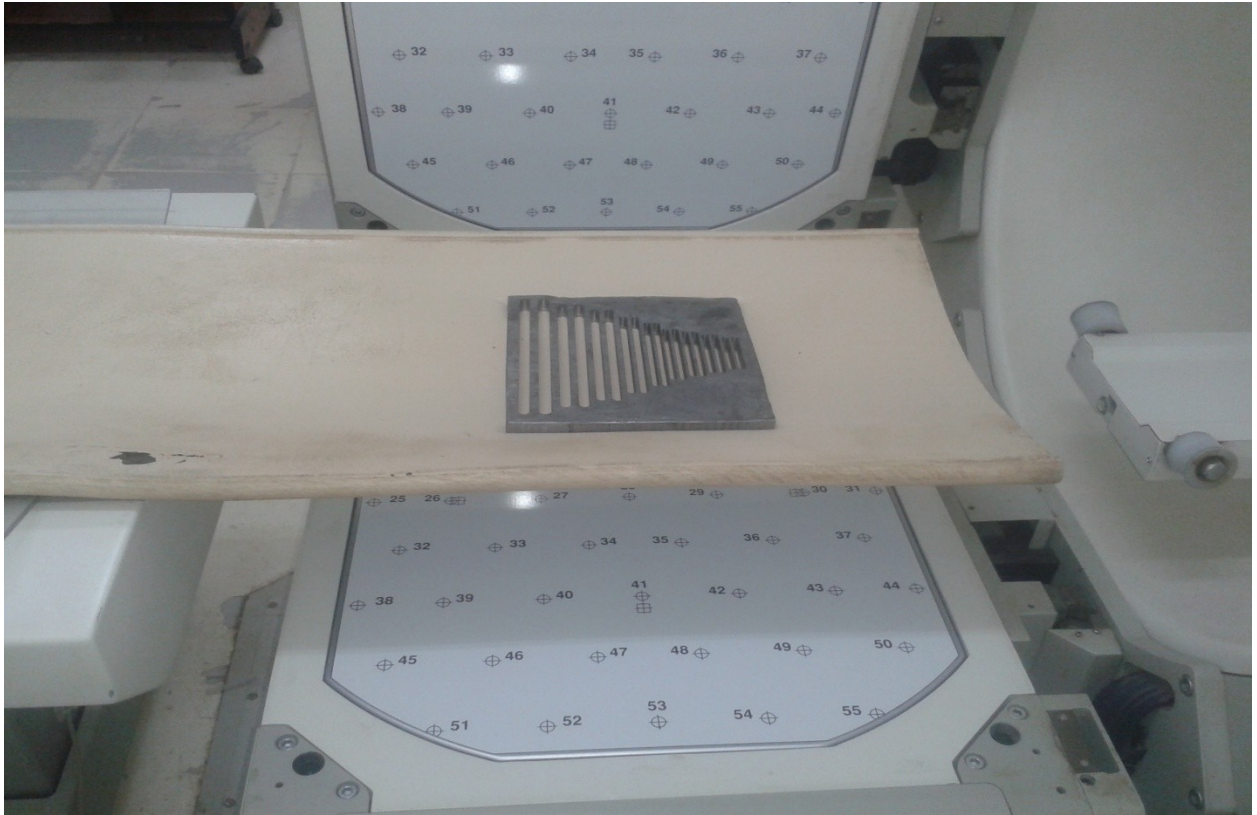
Figure 3-42: Image show the slit phantom centred during intrinsic image
