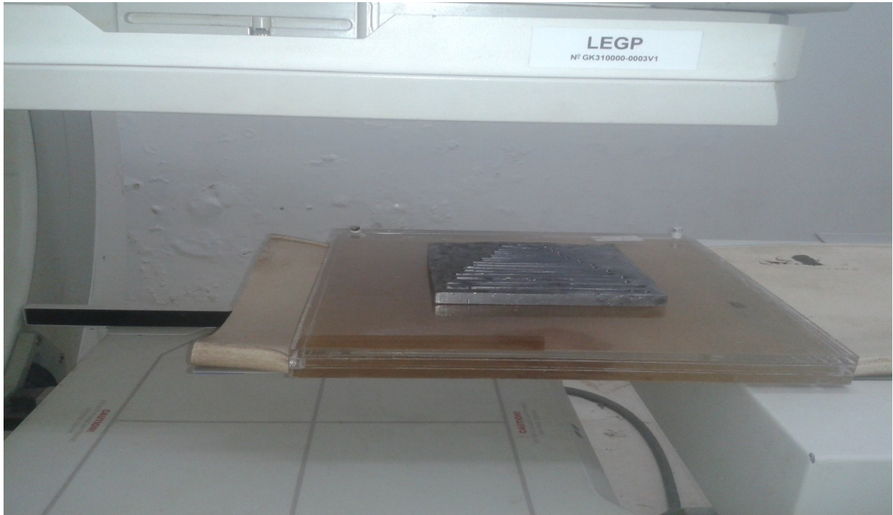
Figure 3-41: Image show the slit phantom and flood phantom during acquisition
