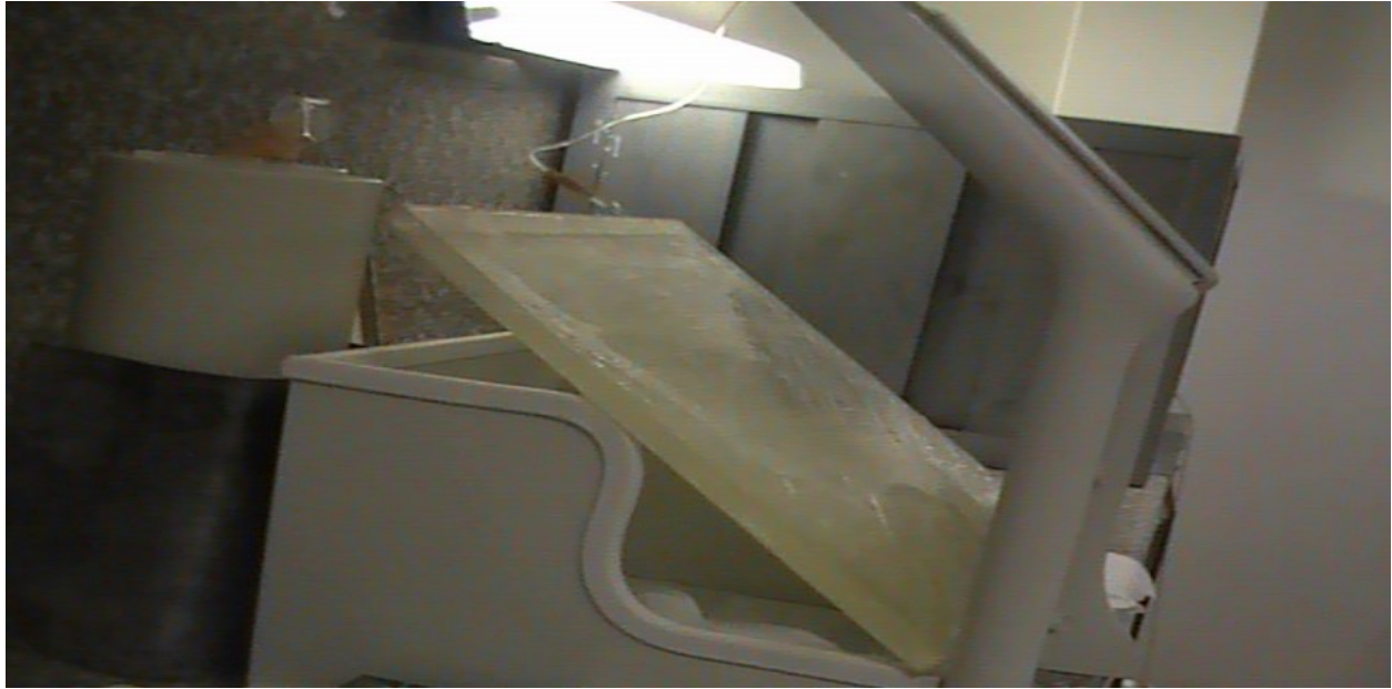
Figure 3- 8: image show the flood phantom during filling with water (side view)
