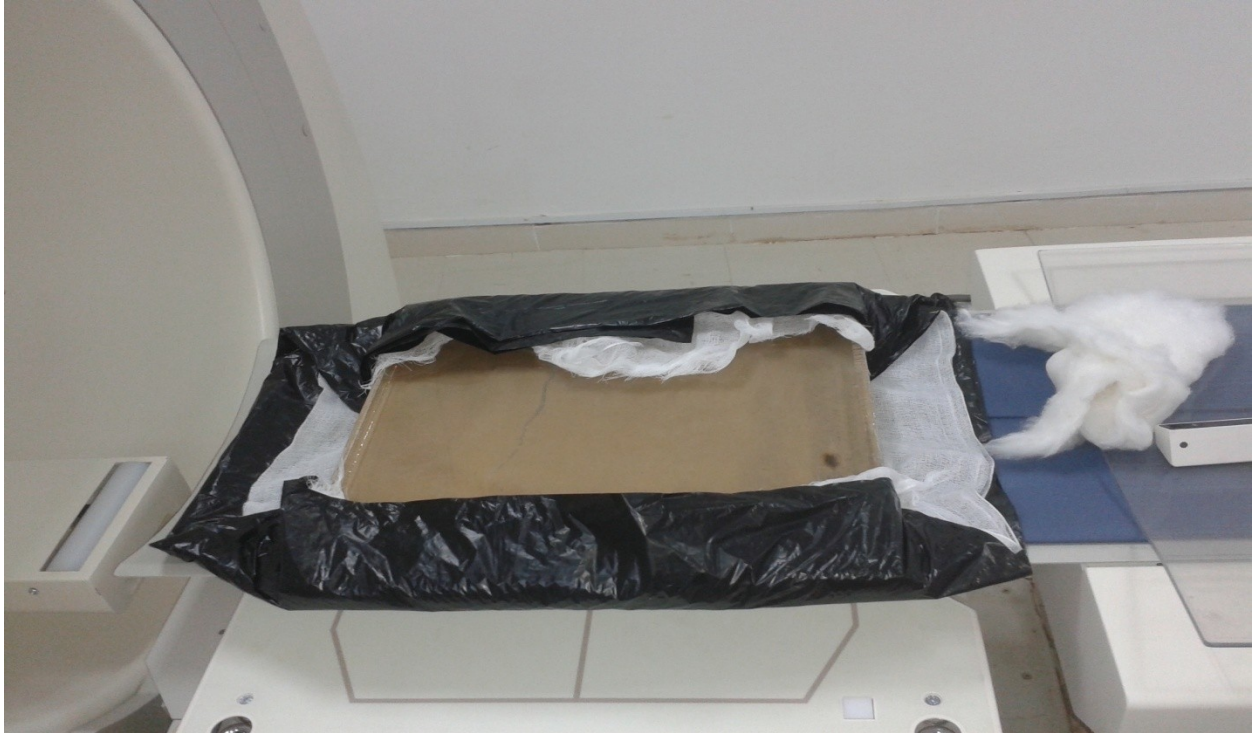
Figure 3-28: image shows the flood phantom center on the camera table with collimator inferior
