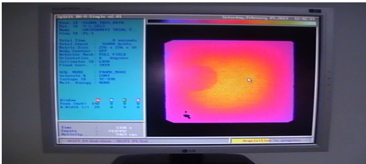
Figure 3-13: image show the workstation during uniformity quality control test acquisition
