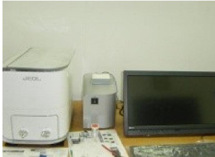
Figure 3.4 JCM-6000 NeoScope Benchtop SEM
