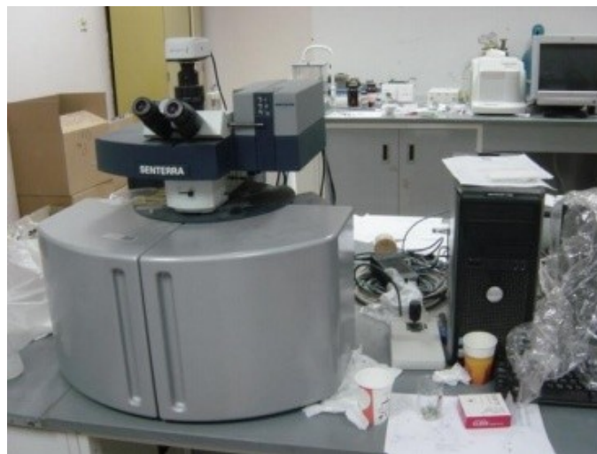
Figure3.5 SENTERRA Raman spectrophotometer
