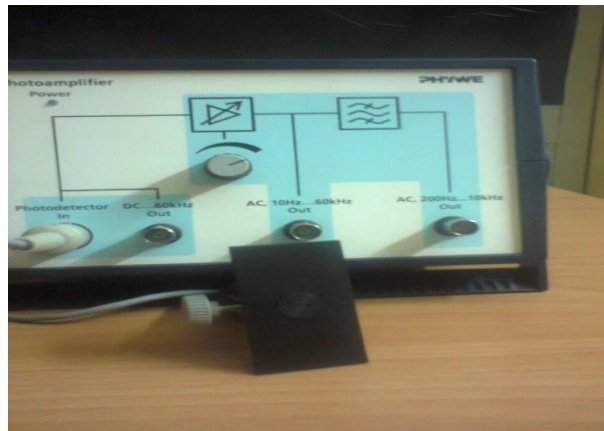
Figure (3.7): photograph of the photoamplifier detector
