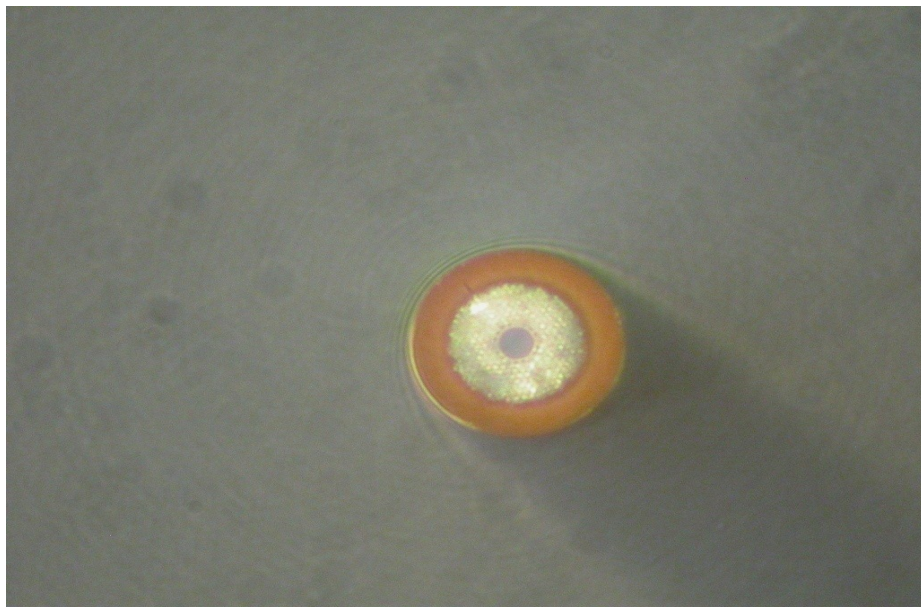
Figure (3.4): The cross section of HC- PCF
