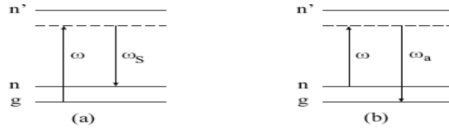
Figure (1.5): Energy level diagrams shows (a) Raman Stokes scattering and (b) Raman anti-Stokes scattering(Birks et al,2004).
