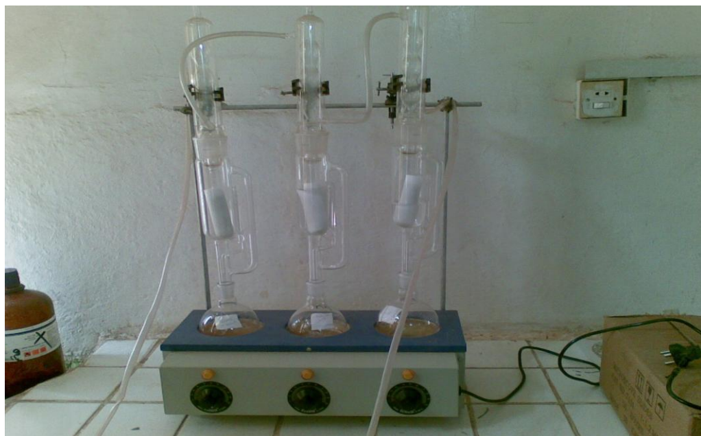
Plate. 7: Soxhlet Extractor Apparatus
