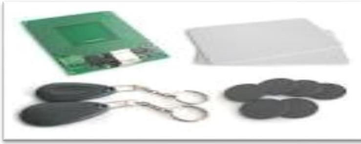
(Figure 2.5): Different types of segments of RFID
