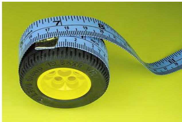
Figure 2-7 Measuring wheel circumference with a cloth tape measure
