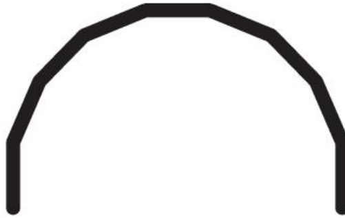
Figure 2-4 Acceptable 180° turn made gradually from 22.5° segments
