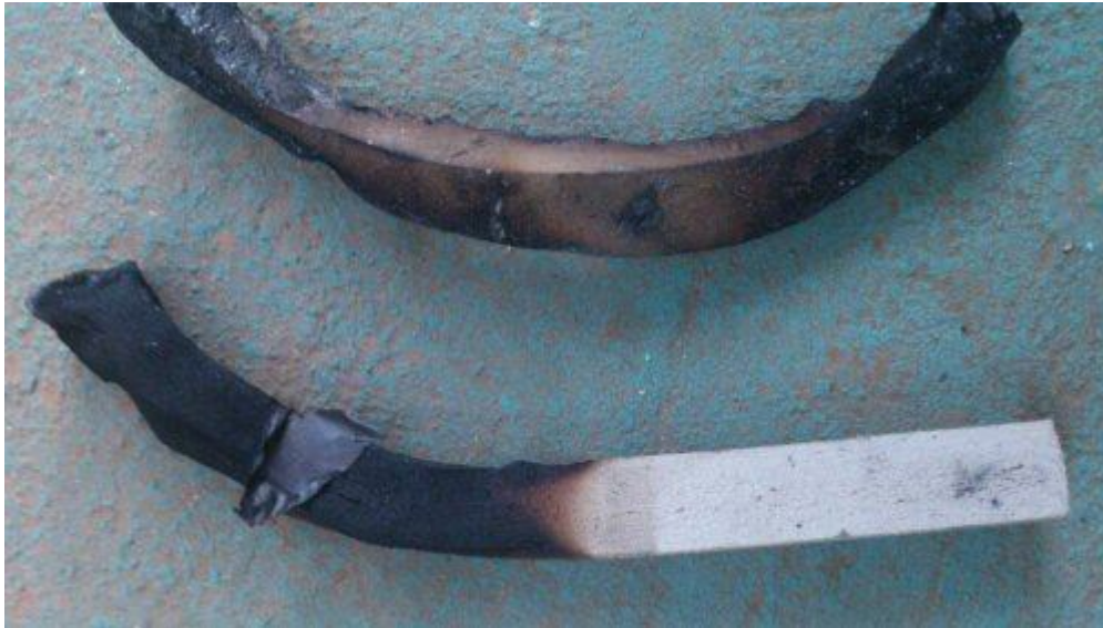
Figure(3.5): WPCs samples after burning
