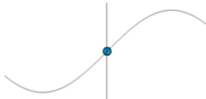
*Figure 2-5 Sinusoidal waves correspond to simple harmonic motion.*
