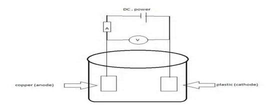
After the preparation of the electrolytic cell systematic process were carried out to study the different operating condition (pH ,concentration, current value) were studied .
