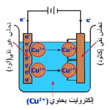
• Process of electroplating deposition :
