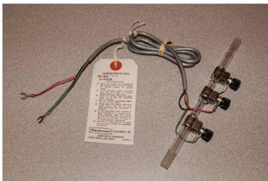
Figure 3.2 Direct-contact style of conductivity probe
