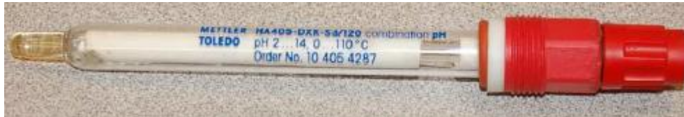
Figure 3.9: Typical industrial combination PH electrode
