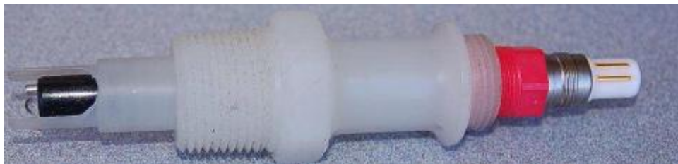
Figure 3.10: PH probe without protective plastic cap covering the probe connector to view gold-plated connector bars
