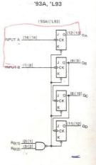
. . . dynamic input activated by transition from a high level to a low level
