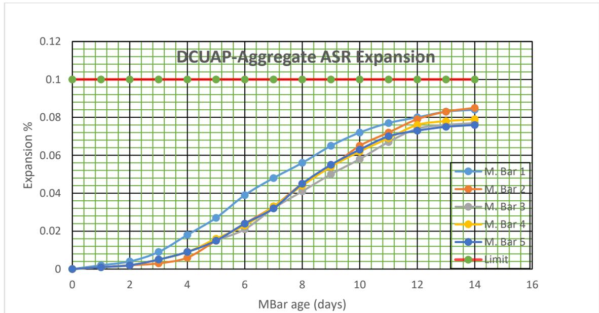
Fig 3.7 Test results of five bars of crushed sand from JAQ mixed with OPC cement of 0.71 - 0.75% Na<sub>2</sub>OE ASTM C1260 accelerated method.
