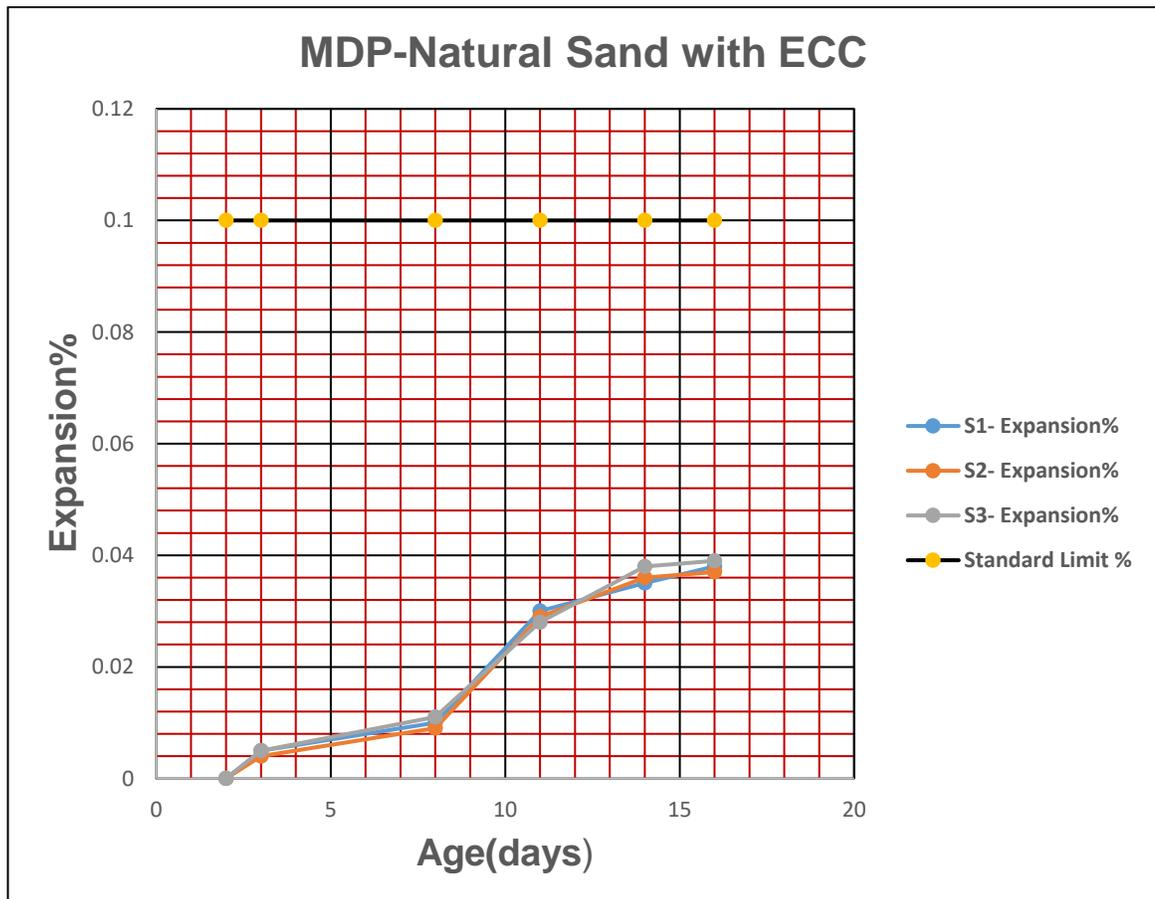
Fig 3.3: Test one natural sand mixed with ECC cement of 0.64% Na<sub>2</sub>Oe (Merowe Dam Project Final Test Report on Concrete LI, Germany, 2009).
