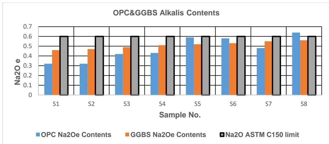
Fig. 4.1 Alkalis Contents in OPC and GGBS Cements compare to ASTM C 150 requirement.
