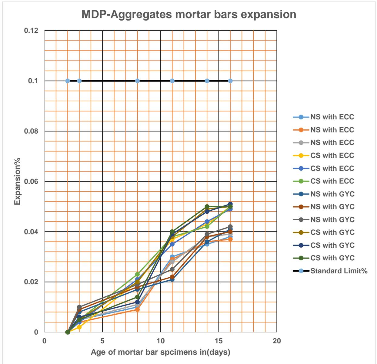
Fig 4.2 Expansion of mortar bars made with Crushed Sand (CS) UDQ source, Natural Sand(NS) Abu Sibba source and ECC & GYC - ASTM C 1260 Accelerated Method.
