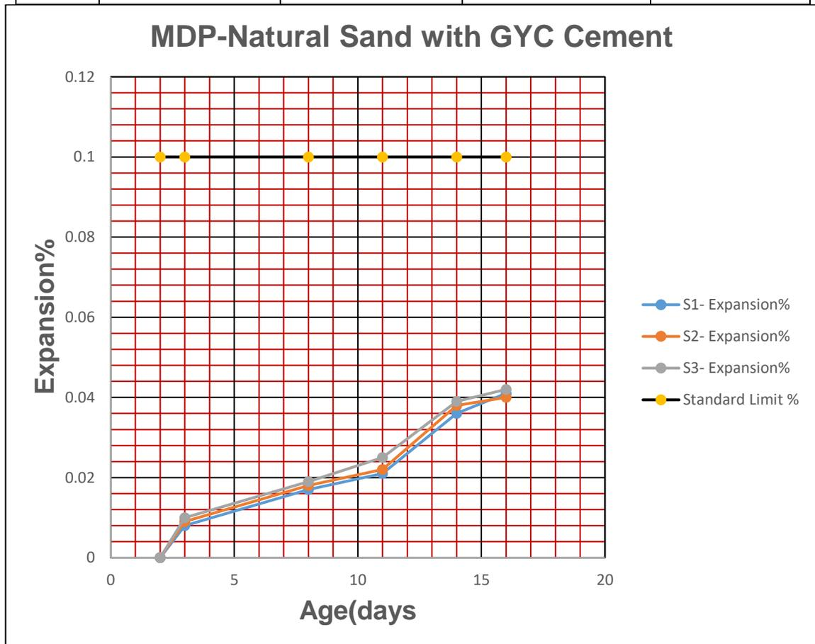
Fig3.5: Test three natural sand mixed with GYC cement of 0.48% Na<sub>2</sub>Oe (Merowe Dam Project Final Test Report on Concrete LI, Germany, 2009. ASTM C 1260 Accelerated Method.
