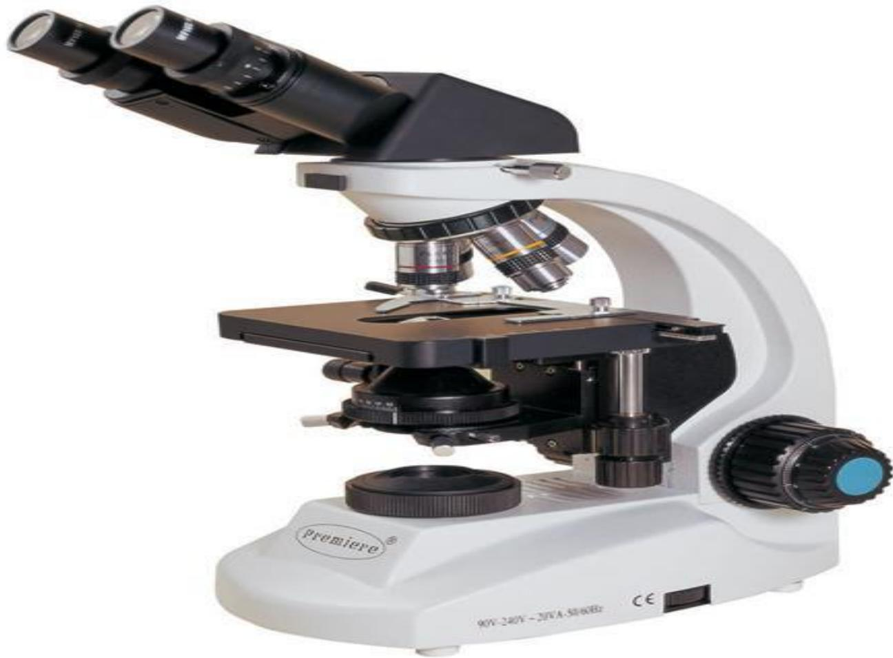
Photo B-8, A petrographic microscope instrument
