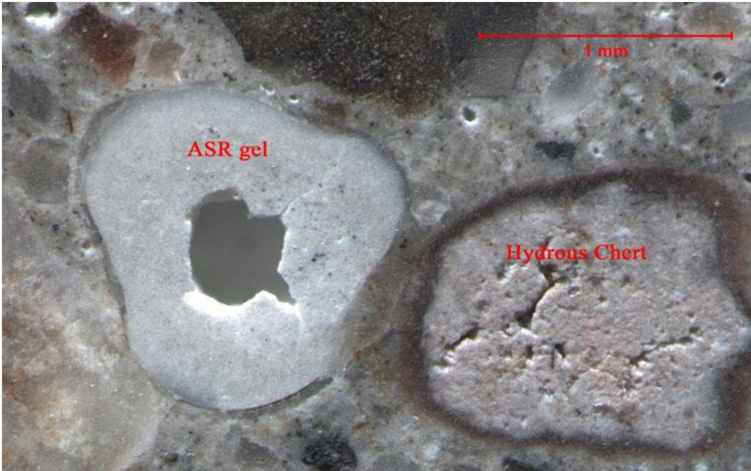
Photo B-11 (ASR) remains a major durability issue affecting concrete structures, including heavy civil infrastructure, such as dams, bridges and pavements
