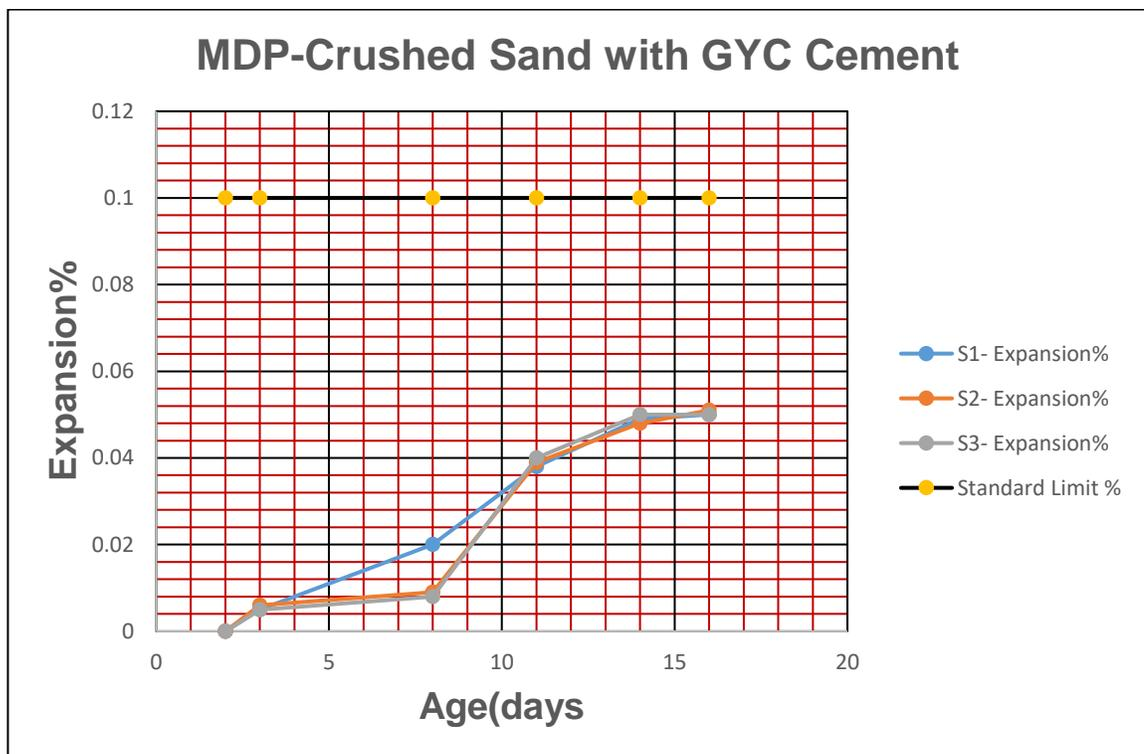
Fig3.6 Test four crushed sand mixed with GYC cement of 0.48% Na<sub>2</sub>Oe (Merowe Dam Project Final Test Report on Concrete LI, Germany, 2009. ASTM C 1260 Accelerated Method.
