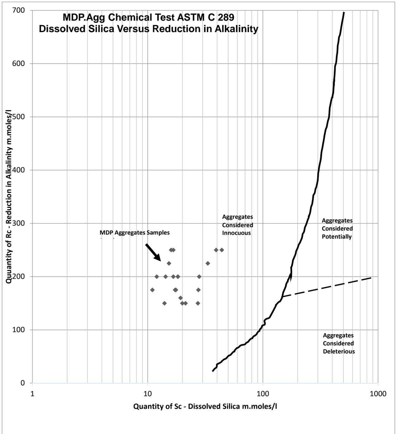
Fig 3.1A Position of the aggregate samples tested in the diagram Sc versus Rc according to ASTM C 289 Standard Evaluation Curve, Chemical Method.
