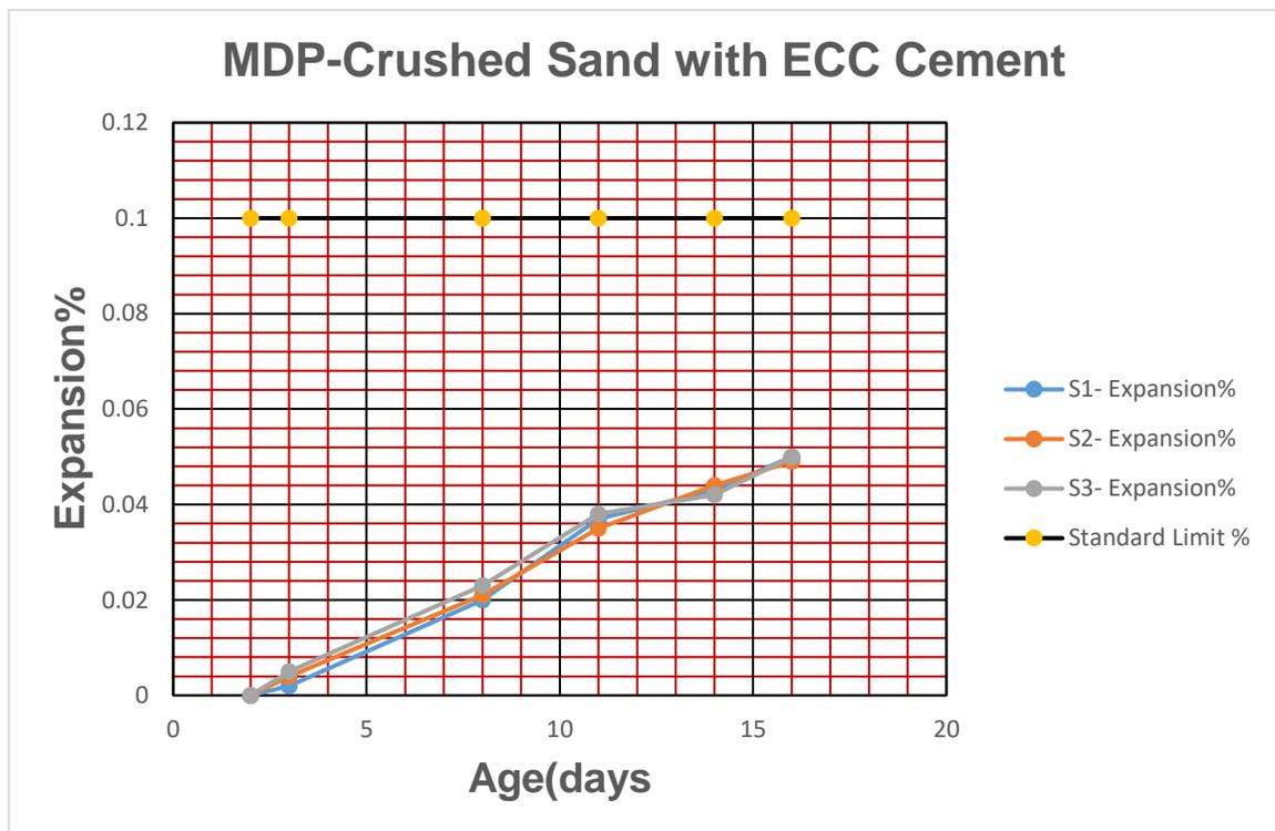
Fig3.4: Test two crushed sand mixed with ECC cement of 0.64% Na<sub>2</sub>Oe (Merowe Dam Project Final Test Report on Concrete LI, Germany, 2009. ASTM C 1260 Accelerated Method
