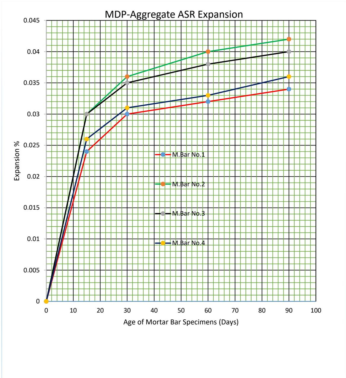
Fig 3.2 expansion of mortar bars subjected to the ASTM C 227 test over a 3-month period using OPC of 1.21% sodium oxide equivalent and Umm Dewiema quarry crushed aggregate (Merowe Dam Project, Concrete Trial Mixes, Test Report CCMD, 2004).
