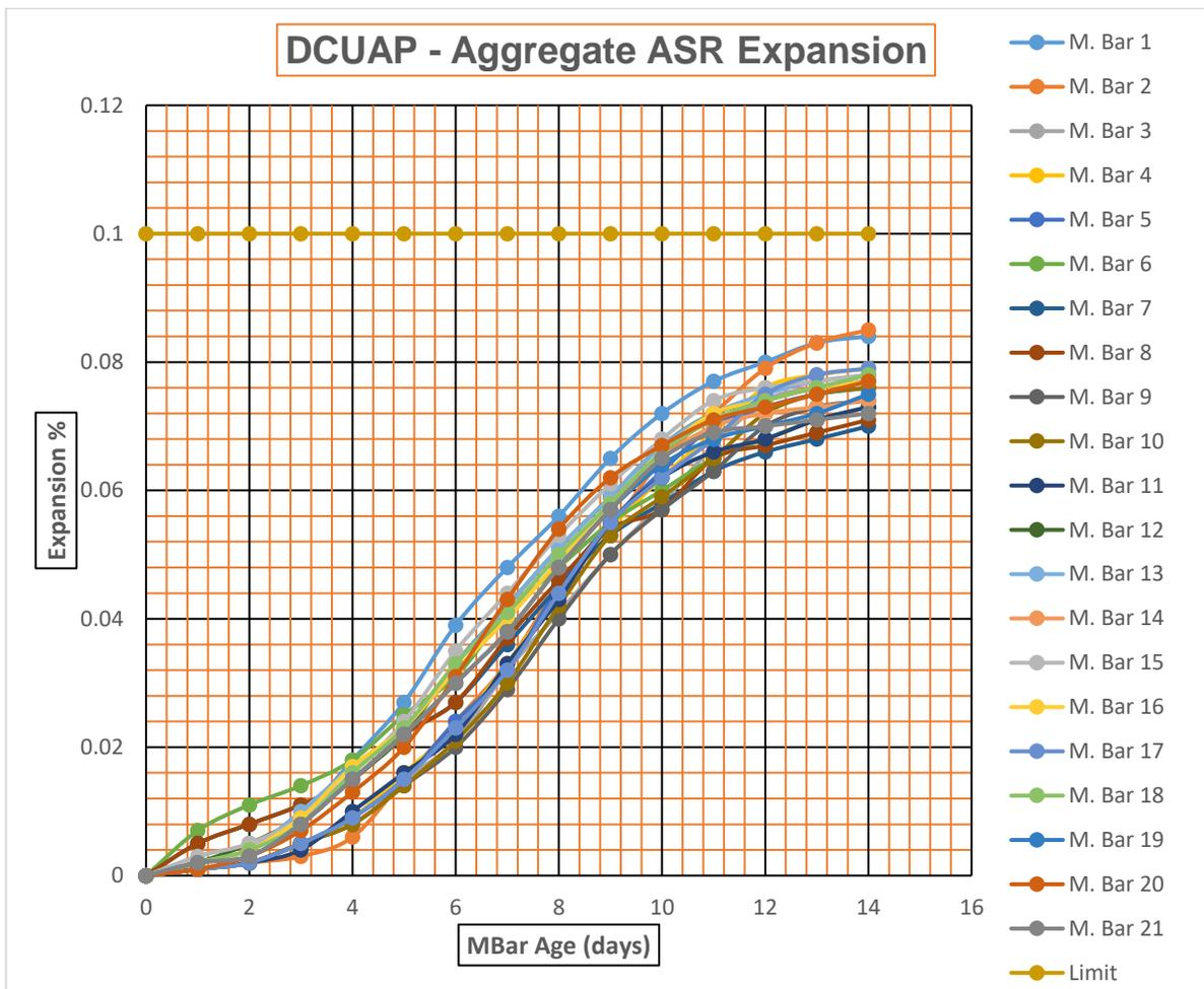
Fig4.3: Expansion of mortar bars from aggregate JAQ source and OPC cement of 0.71 to 0.75% Na<sub>2</sub>OE ASTM C 1260 Accelerated Method (time:2013 to 2017)
