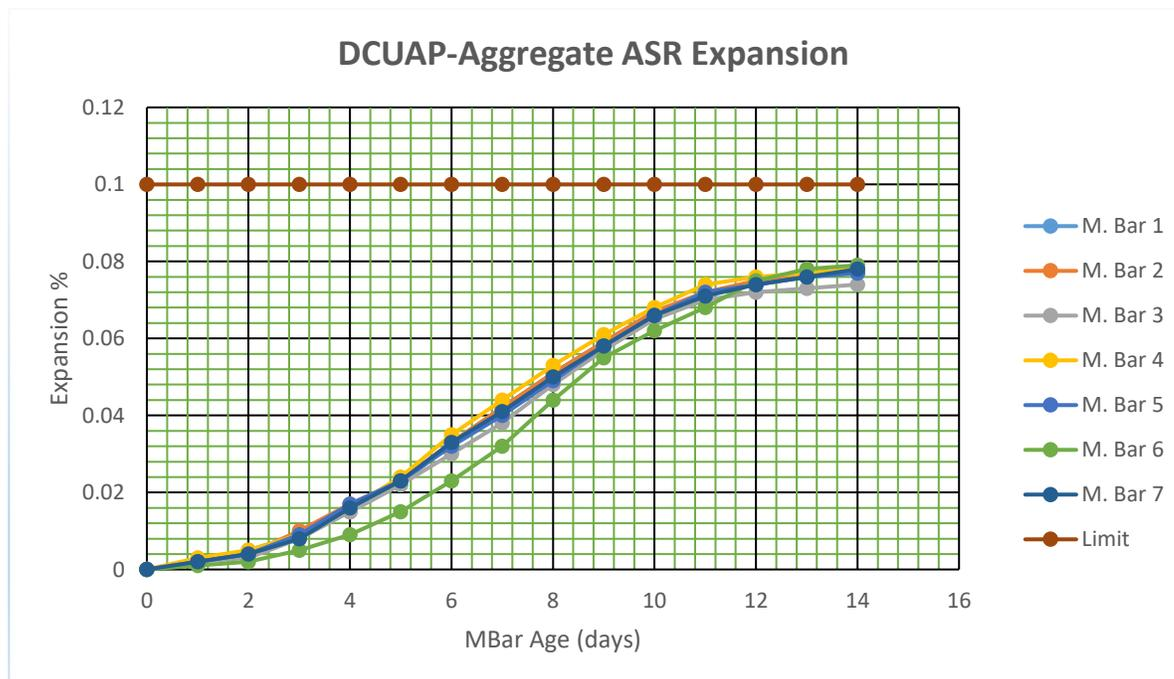
Fig3.9 Test results of seven bars of crushed sand from JAQ mixed with OPC cement of 0.71% Na<sub>2</sub>O<sub>e</sub> ASTM C1260 accelerated method.
