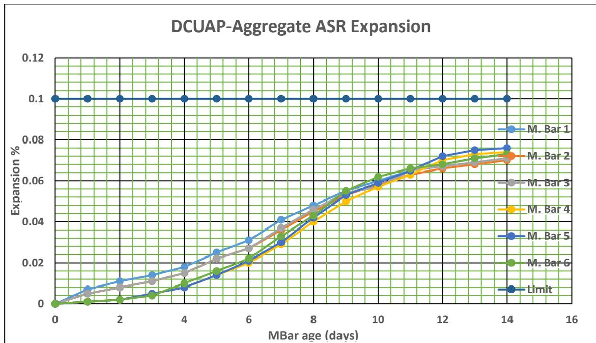
Fig 3.8 Test results of six bars of crushed sand from JAQ mixed with OPC cement of 0.71 - 0.75% Na<sub>2</sub>O<sub>E</sub> ASTM C1260 accelerated method.
