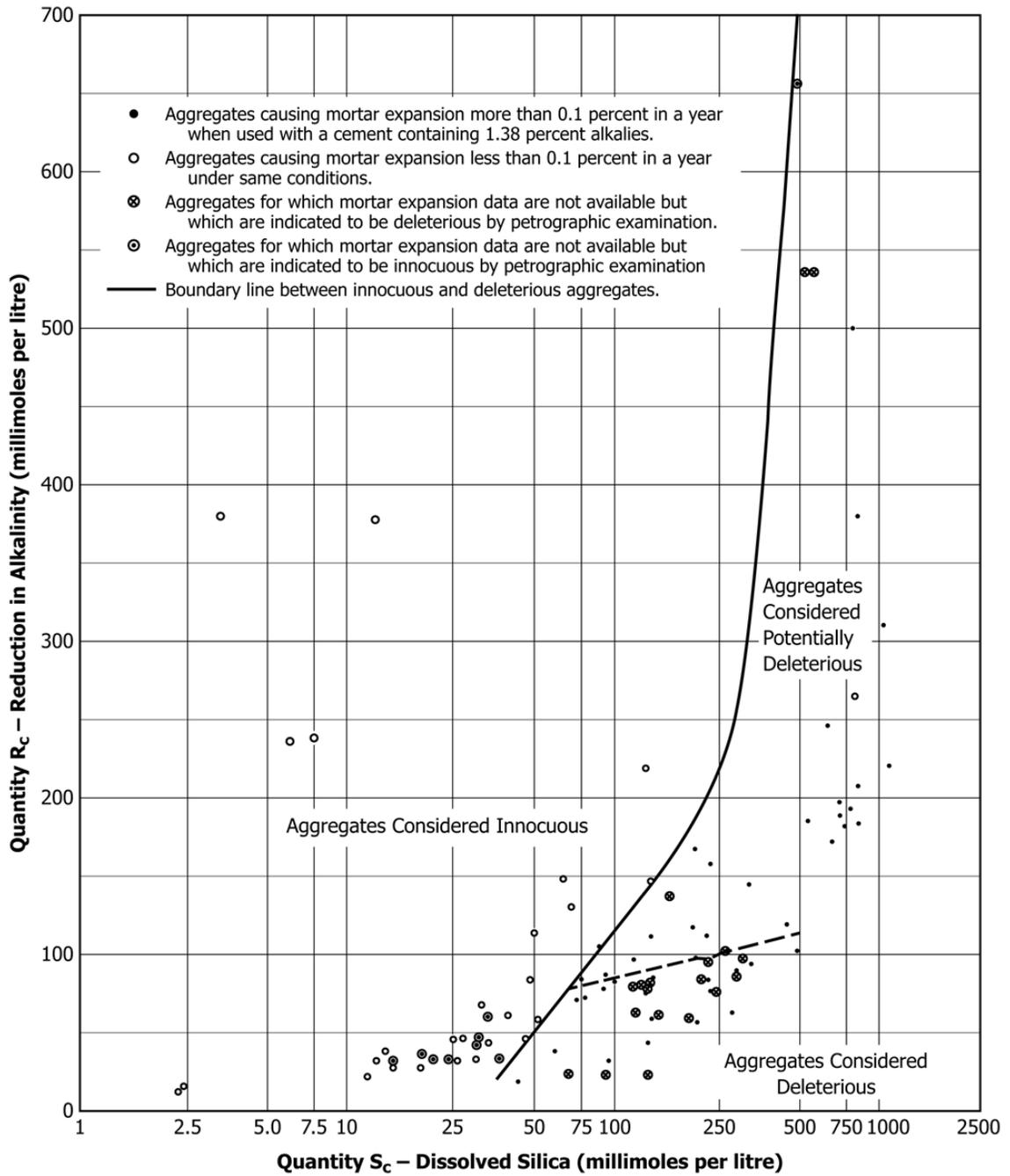
Fig 3.1B ASTM C 289 Standard Evaluation Curve, Chemical Method.
