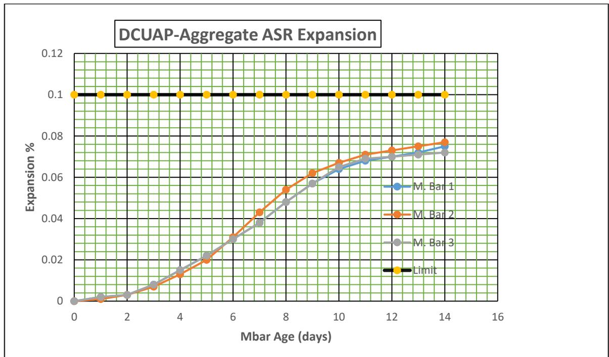
Fig3.10 Test results of three bars of crushed sand from JAQ mixed with OPC cement of 0.75% Na<sub>2</sub>O<sub>e</sub> ASTM C1260 accelerated method.
